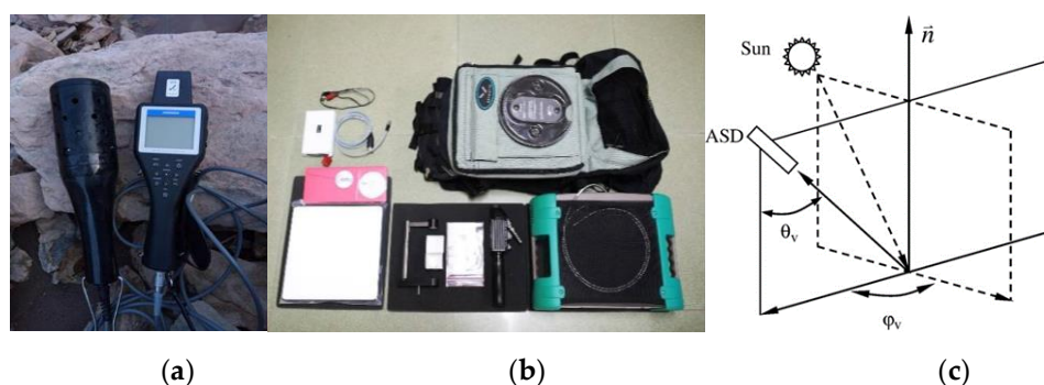
Figure 2. Measuring instrument and Spectrometric method. (a) HORIBA multi-parameter water quality meter U-50; (b) ASD FieldSpec Spectroradiometer; (c) Above-surface observation method [32], where \theta_v is the angle between the observing plane and water surface, and the range of \theta_v is 30–150°; \varphi_v is the angle between the observing plane and the plane of the incident radiation away from the sun, and the range of \varphi_v is 90–135°.
