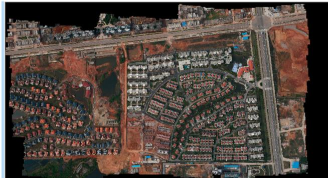
Figure 10. Digital orthophoto map (DOM) generate.
