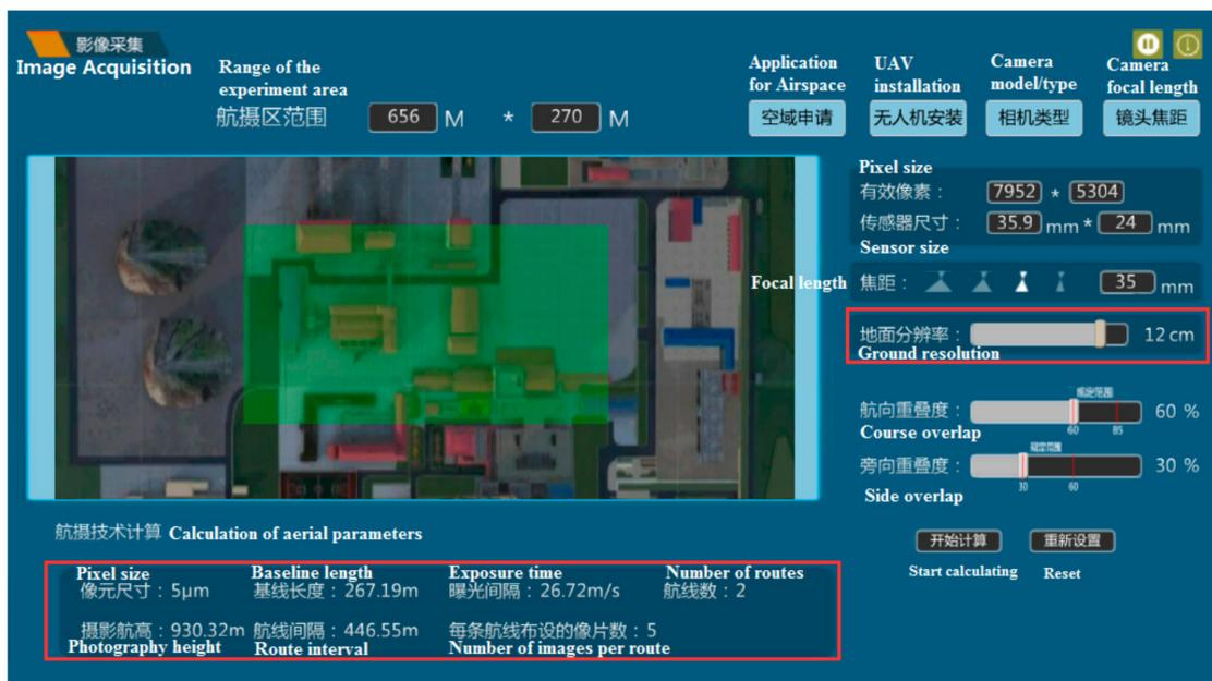
Figure 6. VSETP-UAV Aerial photography parameter selection and calculation.
