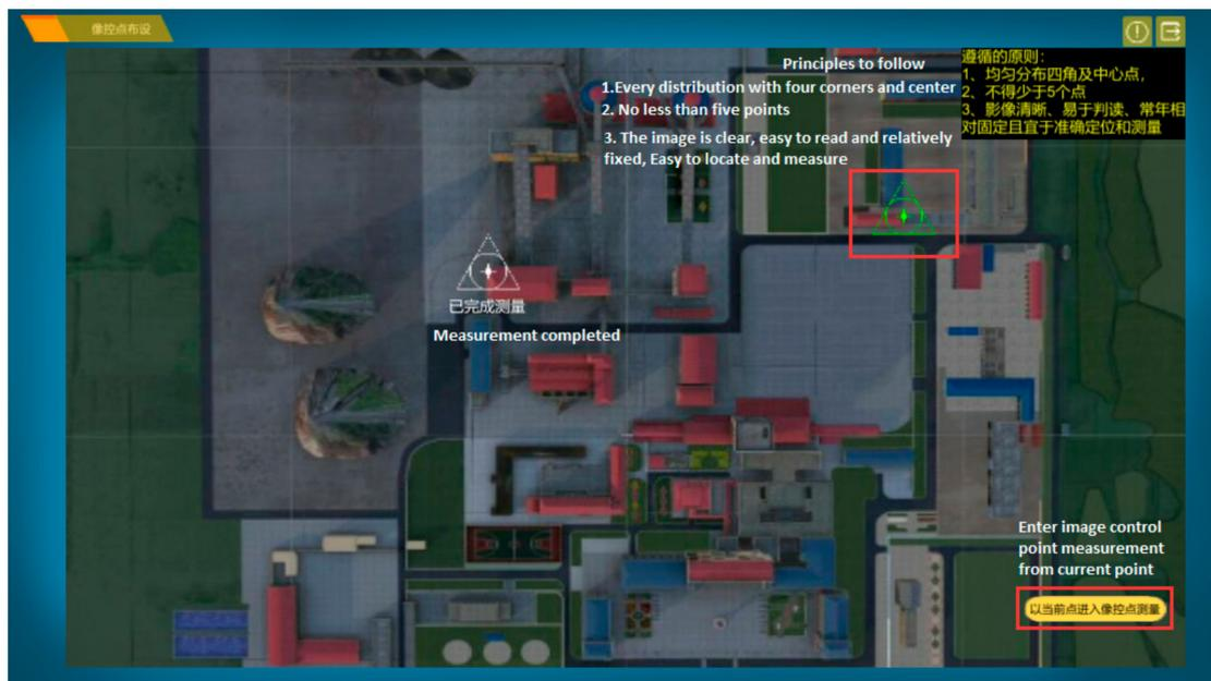
Figure 7. VSETP-UAV Layout of image control point.
