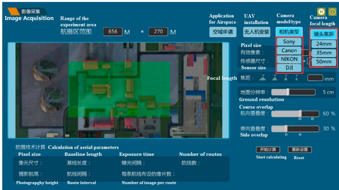
Figure 5. VSETP-UAV Camera Parameter Setting.
