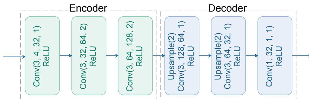
Figure 2. The pretrained AutoEncoder for feature loss calculation.
