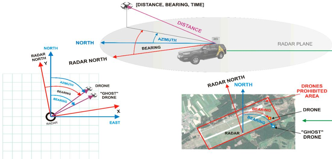
**Figure 3.** An example of drone misclassification due to a large azimuth error. The radar indicates "GHOST DRONE" (blue rectangle with a white background), and the system classifies it as an object that does not violate the airport zone. In fact, "DRONE" (red rectangle with a yellow background) violates the forbidden zone.
