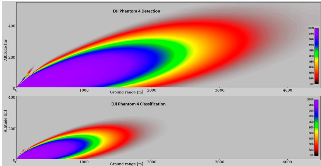
**Figure 2.** DJI Phantom 4 drone detection (upper) and classification (lower) ranges for one of FMCW radars available on a commercial market (the characteristics were obtained from the manufacturer, who asked not to disclose the name and model of the radar for obvious reasons).
