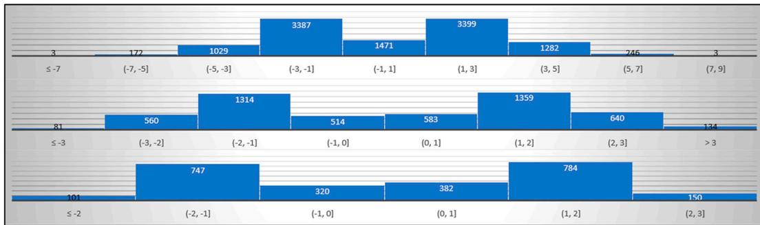
**Figure 13.** Histogram of initial (before calibration) errors of the R1 radar orientation in the 4-radars system, for which the azimuth misalignment increased after calibration: above 0%(upper), above 50%(middle), and above 100%(lower).
