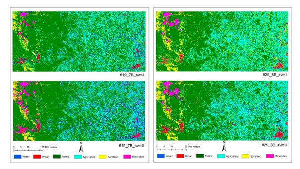
Figure 4. Classification method I and II with 2000 and 2017 images used dataset (B) with SVM algorithm.
