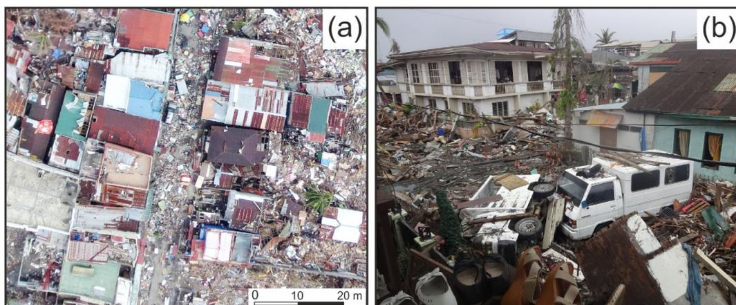
**Figure 7.** Debris and rubble deposited by the typhoon and the storm surge in the areas near the coast, in (a) Tacloban, and (b) Basey (Samar), masking the actual structural damage. The UAV/drone image in (a) also demonstrates the additional level of detail such data can provide. Sources: (a) Corephil/OpenAerialMap, and (b) L. Ruiz/Wikipedia, CC BY-SA 4.0.
