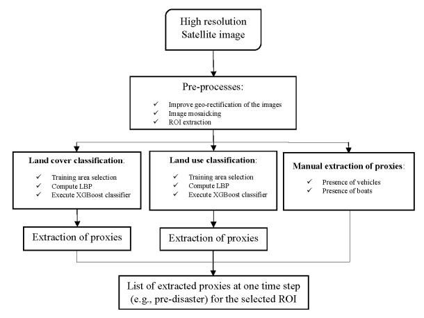
**Figure 3.** Framework for the extraction of proxies using high resolution satellite images for each region of interest (ROI) at each time step (e.g., pre-disaster, T0).
