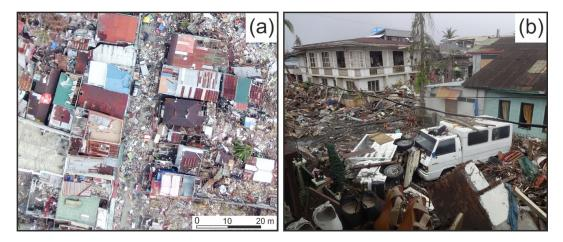
**Figure 7.** Debris and rubble deposited by the typhoon and the storm surge in the areas near the coast, in (**a**) Tacloban, and (**b**) Basey (Samar), masking the actual structural damage. The UAV/drone image in (**a**) also demonstrates the additional level of detail such data can provide. Sources: (**a**) Corephil/ OpenAerialMap, and (**b**) L. Ruiz/Wikipedia, CC BY-SA 4.0.
