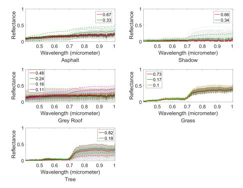
**Figure 8.** The wavelength reflectance space of the endmember signature estimated for the Gulfport dataset, which has the same meaning as in Figure 5.
