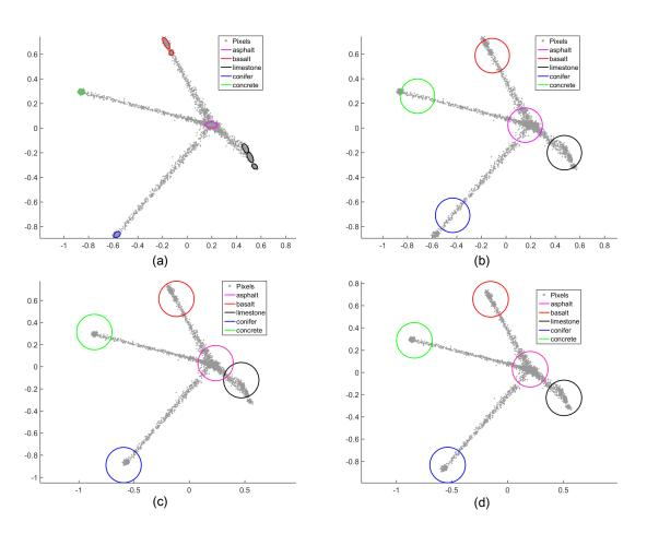
**Figure 14.** The scatter plot of the synthetic dataset under different initial conditions. The gray dots are the pixels when projected by PCA. (**a**) The original endmember scatter plot of the synthetic dataset with estimated GMM. (**b**) The endmember scatter plot by K-means initialization. (**c**) The endmember scatter plot by VCA initialization. (**d**) The endmember scatter plot by region-based VCA initialization.
