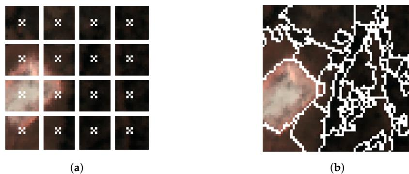
**Figure 7.** SLIC segmentation for region size initially set to  $16 \times 16$ : (a) initialization stage; (b) final segmentation.
