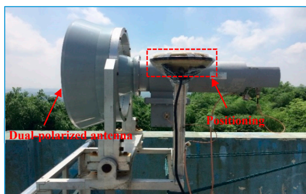
Figure 1. Outdoor antenna section of the Global Navigation Satellite System (GNSS) dual-polarized rain detection system.
