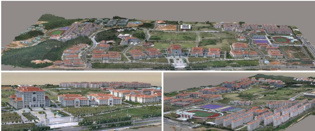
**Figure 5.** The generated 3D image-based point cloud of the Xiangan campus of Xiamen University.
