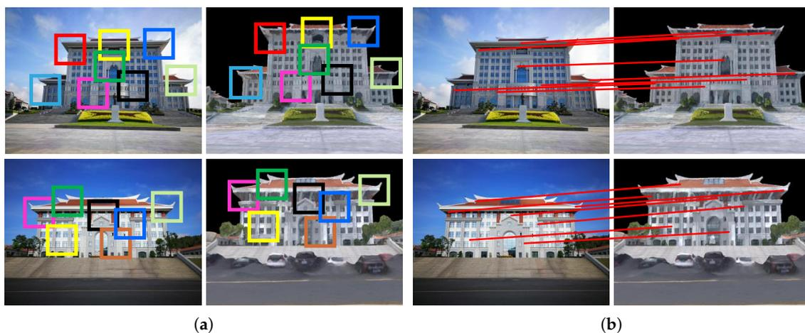
**Figure 14.** Cross-domain image patch matching results and center point connection of matching image patches. Left: Ground camera images; Right: Rendered images with the same viewpoint of ground camera image. (a) Cross-domain image patch matching results. (b) Center point connection of the matching image patches in (a).
