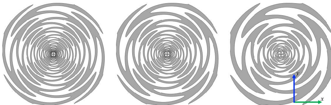
Figure 1. Sinuous antennas having parameters: P = 20 cells, \tau = 0.8547 (left); P = 16 cells, \tau = 0.8228 (center); and P = 12 cells, \tau = 0.773 (right). Other parameters constant for all antennas: N = 4 arms, R_T = 10 cm, R_{in} = 0.4 cm, \alpha = 45^\circ , and \delta = 22.5^\circ .
