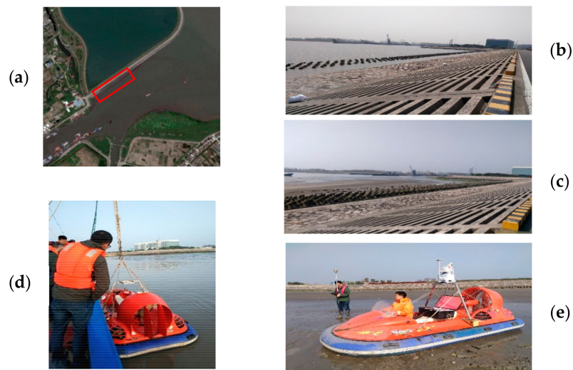
Figure 6. (a) The test mudflat zone (b) during high tide, (c) during low tide. (d) Lifting the equipment; (e) Topographic survey.
