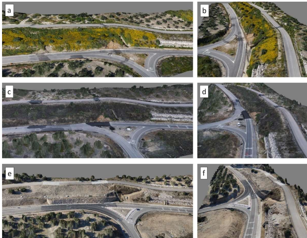
Figure 2. (a) Photorealistic reconstructions of the landslide foot with the roads affected: (a): 24 April 2013 frontal view; (b): 24 April 2013 lateral view; (c): 5 March 2014 frontal view; (d): 5 March 2014 lateral view; (e) 19 November 2015 frontal view; (f): 19 November 2015 lateral view (it can be observed the drainage wells and the retaining wall).
