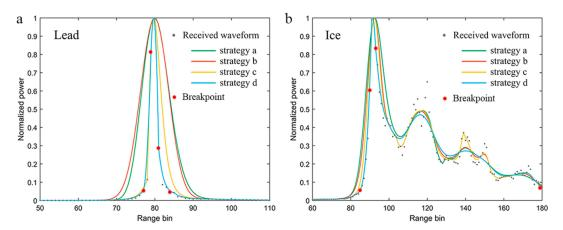
**Figure 2.** Comparisons of fitting performances using segment strategy a, strategy b, strategy c, and strategy d for typical lead (**a**) and ice (**b**) waveforms. Red points are the breakpoints for strategy d.
