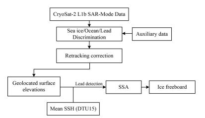
**Figure 3.** Flowchart of the CS-2 ice freeboard retrieving algorithm. Here, SSH is sea surface height and SSA is sea surface height anomaly, respectively.
