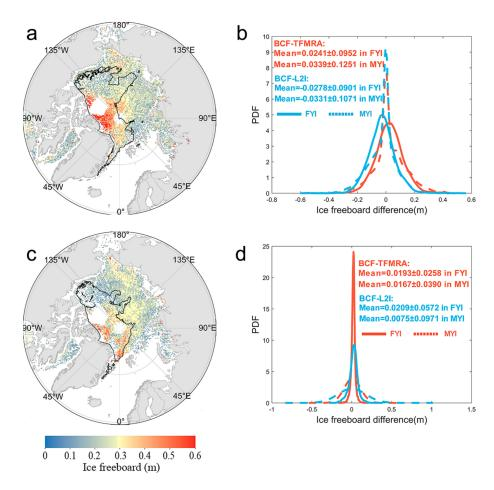
**Figure 5.** Ice freeboard from BCF (**a** and **c**), probability density function of ice freeboard difference between BCF and TFMRA, BCF and CS-2 L2I products in March 2015 (**b**) and April 2016 (**d**). The black polygon defines the extent of the MYI zone.
