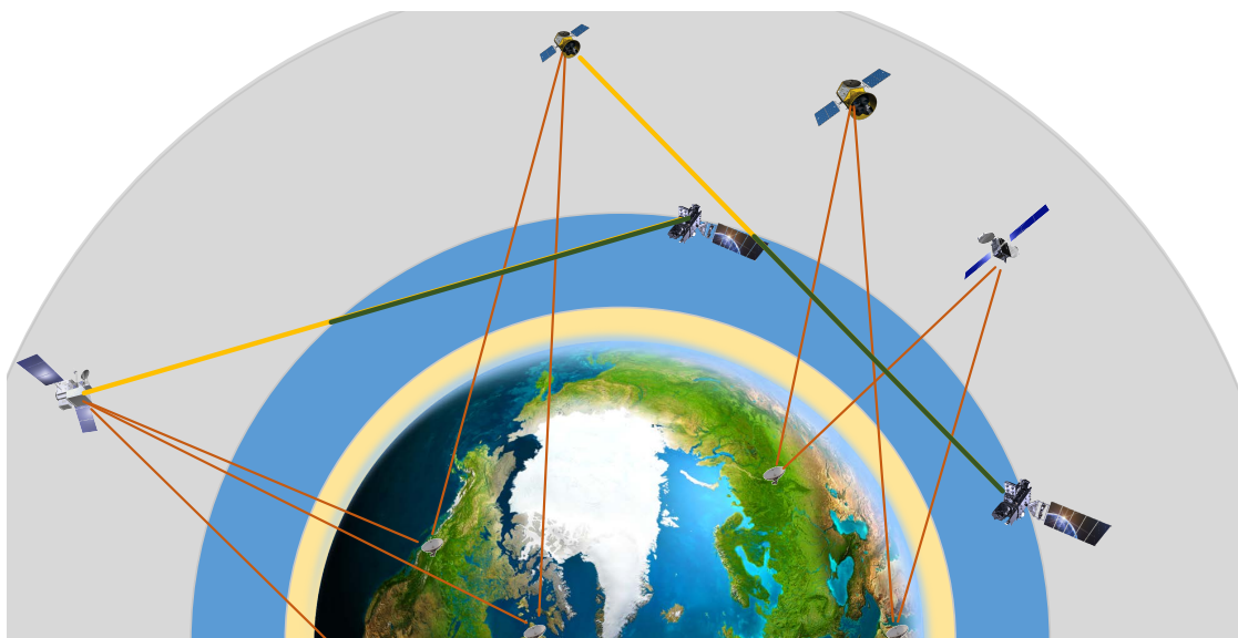
Figure 1. Multiobserving systems: green line, signal path across bottom region of the ionosphere 800 km during occultation; yellow line, signal path across the top region during occultation; and orange line, signal path across the ionosphere of ground-based GNSS observation.
