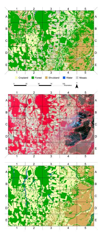
**Figure 4.** Comparison of GlobCover 2009 (**top**), Landsat 5 (**middle**) and BULC-U 2009 (**bottom**), showing the coarse resolution of GlobCover, the increased level of spatial detail available with Landsat, and the resulting BULC-U 2009 image created by fusing Landsat imagery and GlobCover 2009. The Landsat image is from 12 September 2010.
