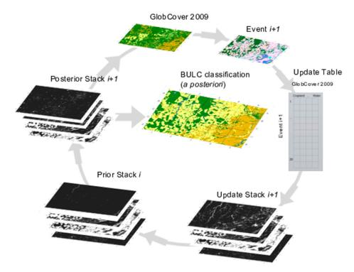
**Figure 2.** Schematic of BULC-U. The BULC-U processing is driven by unsupervised classifications and update tables relating them to a common reference classification (here, the GlobCover 2009 classification). As in BULC, evidence from each new Event is used to update the estimates of each pixel's LULC using Bayes' Theorem.
