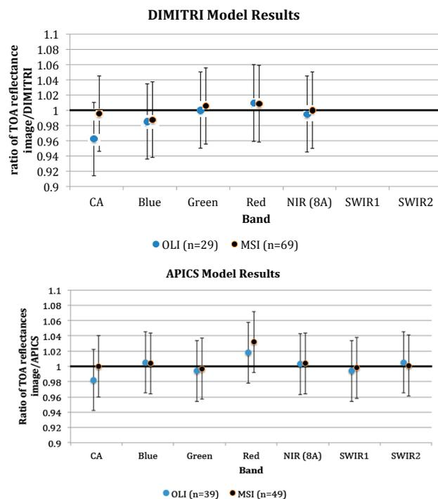
**Figure 9.** Absolute PICS model results for calibration of Landsat-8 OLI and Sentinel-2A MSI for the Libya-4 region. The top figure shows the Database for Imaging Multi-spectral Instruments and Tools for Radiometric Intercomparison (DIMITRI) results for the visible and near-infrared (VNIR) bands (DIMITRI does not include data for the shortwave infrared (SWIR) bands) and the bottom figure shows the APICS results for all the common spectral bands.
