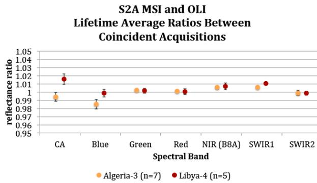
**Figure 8.** The average lifetime ratio between top-of-atmosphere (TOA) reflectances for coincident acquisitions of Landsat-8 and Sentinel-2A for the common spectral bands with 1-sigma error bars. There were seven cloud-free coincident acquisitions for Algeria-3 since the Sentinel-2A launch and five of Libya-4.
