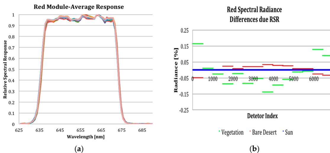
**Figure 1.** (a) Spectral responses of each focal plane module in the OLI red band; (b) effects of spectral response differences in uniformity across the focal plane when flat fielded on the solar diffuser [4].
