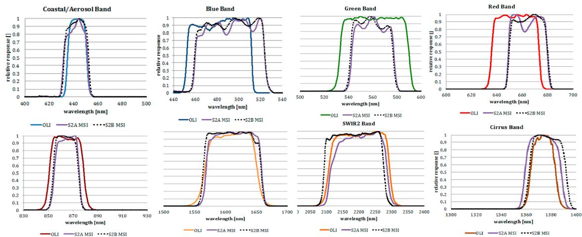
**Figure 7.** Comparison of the spectral response functions for Landsat-8 and Sentinel-2. Even though there is a high degree of similarity among the three instruments, differences require calculation of a spectral band adjustment factor (SBAF) to make data from the three sensors interoperable.
