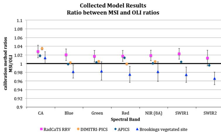
**Figure 11.** The collected absolute calibration results presented as a difference between the instrument ratios for each model. The error bars are a measure of the uncertainty in terms of the standard deviation of the mean.
