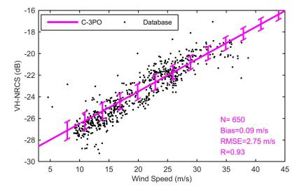
**Figure 2.** C-3PO hurricane wind retrieval model. The magenta line is for the middle incidence angle (34.5°), as well as the bars for the incidence angle ranges (from 19.5° to 49.5°) of the RADARSAT-2 ScanSAR mode.
