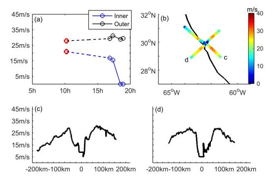
**Figure 6.** ERC dynamic process of Hurricane *Bertha* measured by aircraft SFMR: (**a**) hurricane intensities of the double-eye structure, (**b**) flight tracks, as well as (**c**), (**d**) the respective complete profiles along radius.
