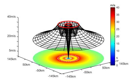
**Figure 3.** An example of the SHEW symmetric double-eye hurricane structure. The maxima wind speeds for two eyes are both 35 m/s, the RMW for the inner core is 15 km and for the secondary core is 45 km, and the two decay parameters are both 0.5.
