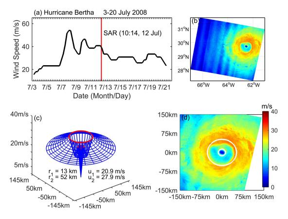
**Figure 5.** Hurricane *Bertha* (2008): (**a**) SAR captured time respective to the time series of Best Track Intensities; (**b**) retrieved sea surface wind speed from SAR images acquired at 10:14 UTC, 12 July 2008; (**c**) SHEW estimated closest idealized structure; and (**d**) storm-centered wind field of hurricane core.
