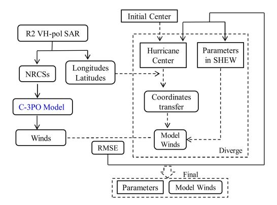
Figure 4. Flowchart for the modified SHEW model to estimate the hurricane double-eye structure.
