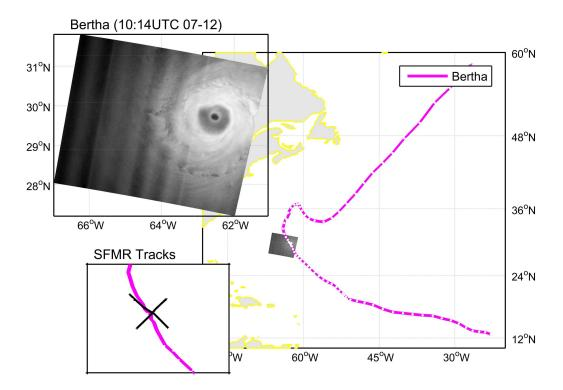
**Figure 1.** VH-polarized SAR image from C-band RADARSAT-2 over Hurricane *Bertha* (10:14 UTC, 12 July 2008), as well as flight tracks of SFMR measurements relative to the same hurricane internal dynamic processes and the Best Track (BT) of Hurricane *Bertha* (2008). RADARSAT-2 Data and Product MacDonald, Dettwiler, and Associates Ltd., All Rights Reserved.
