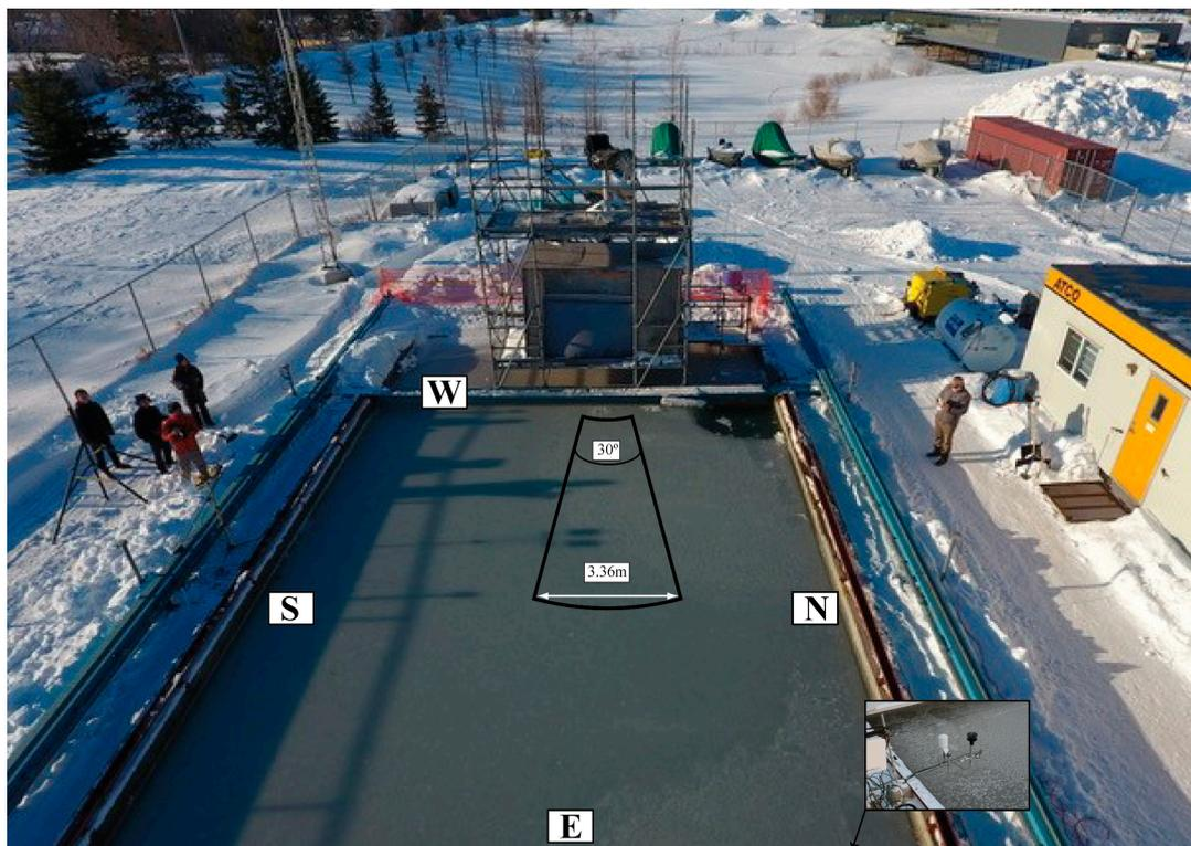
**Figure 1.** The SERF pool located on the University of Manitoba campus. The C-band scatterometer was mounted on the west side of the pool (shown in a stowed protected configuration at the end of the experiment). The LiDAR is located within the protected area beneath the scatterometer. Inset shows the automated meteorological equipment.
