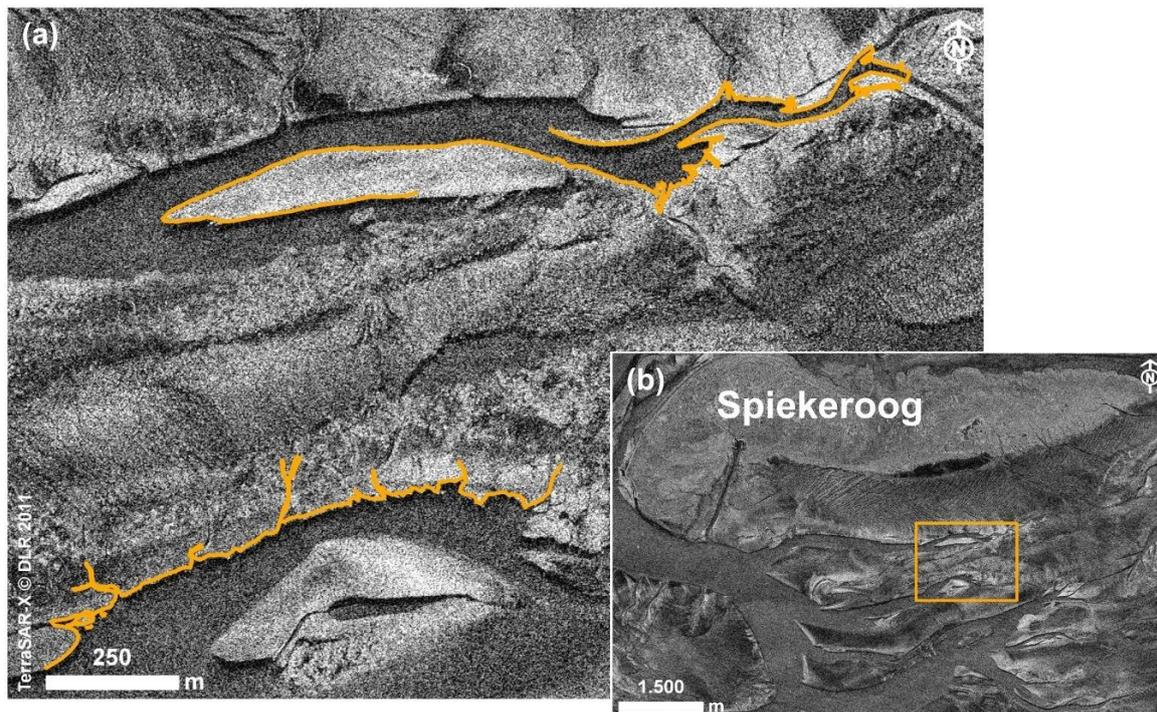
**Figure 2.** In situ verification of land-water-lines: (a) GPS measurement of channel edges synchronous to satellite overflight at 14 min. after low tide (yellow line); (b) location of study area (rectangle) in the tidal flats of Spiekeroog (SL of 17/05/2011, ascending orbit).
