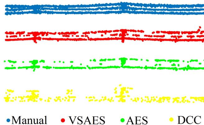
**Figure 8.** Vertical profile of the distribution lines from manually selected raw data and filtered result using the VSAES, AES and DCC methods.
