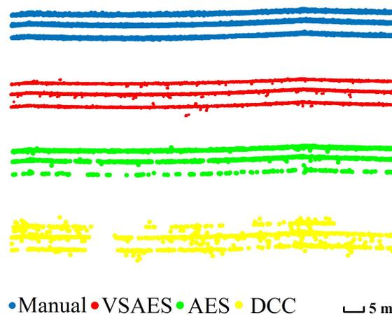
**Figure 6.** Vertical profile of the transmission line from manually selected raw data and filtered results using the VSAES, AES and DCC methods.
