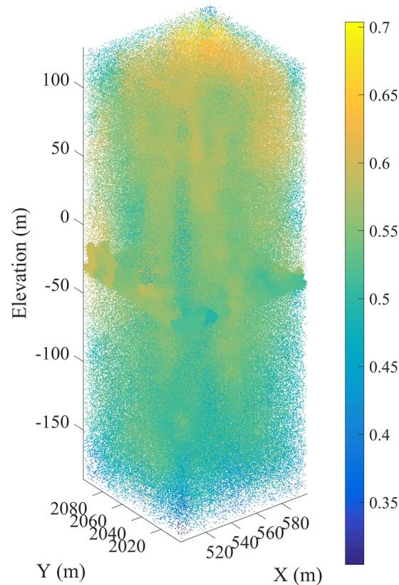
**Figure 4.** Estimated expected number of noise points for a representative voxel using the VS model. The data are colored by the expected number of noise returns.
