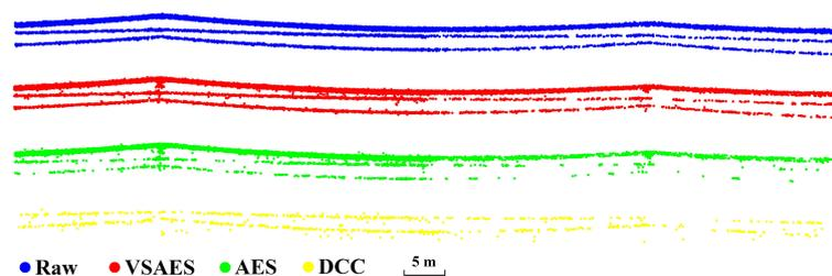
**Figure 10.** Vertical profile of the transmission lines for Lufkin study area from manually classified raw data and filtered results using VSAES, AES and DCC methods.
