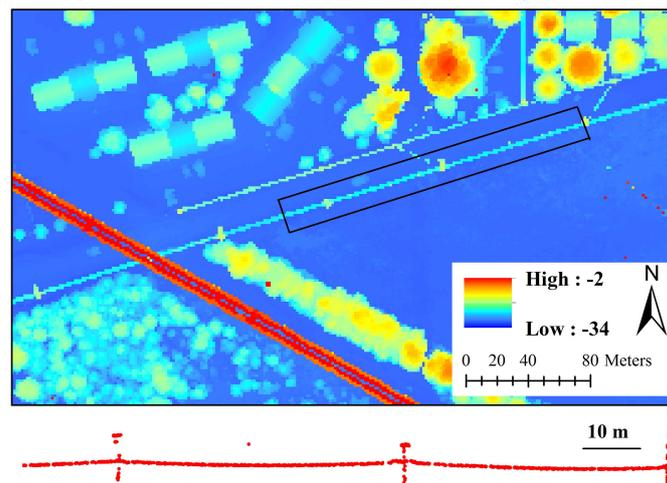
**Figure 12.** Plan and profile view of the Lufkin study area distribution line captured using a Leica ALS-80 linear mode lidar system.
