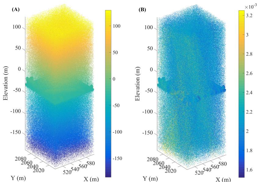
**Figure 2.** An overview of a 100 m × 100 m data block after tiling: (A) colored by elevation; and (B) colored by estimated line point density.
