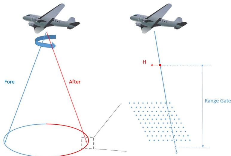
**Figure 1.** An overview of the SPL100 scanning pattern: (left) fore and after observation data; and (right) the details of one laser shot and beamlet vectors. The transmitted laser pulse is split into 100 beamlets and the footprints form a  $10 \times 10$  array on the target. A range gate is used to truncate the raw data. H is the highest point in one beamlet vector, i.e., the start of the range gate.
