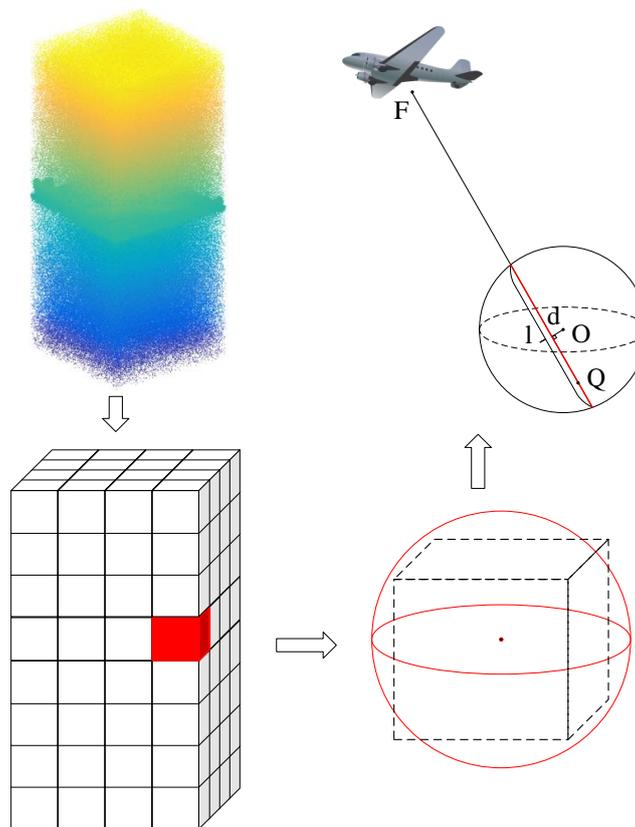
**Figure 3.** Workflow for the VS model. The data block is first voxelized into  $10 \times 10 \times 10$  m voxels. Then, for each point, a sphere with the same volume as the voxel is defined at the center of the voxel. Finally, the expected number of noise points is calculated based on the geometry of the data points and the corresponding aircraft trajectory.
