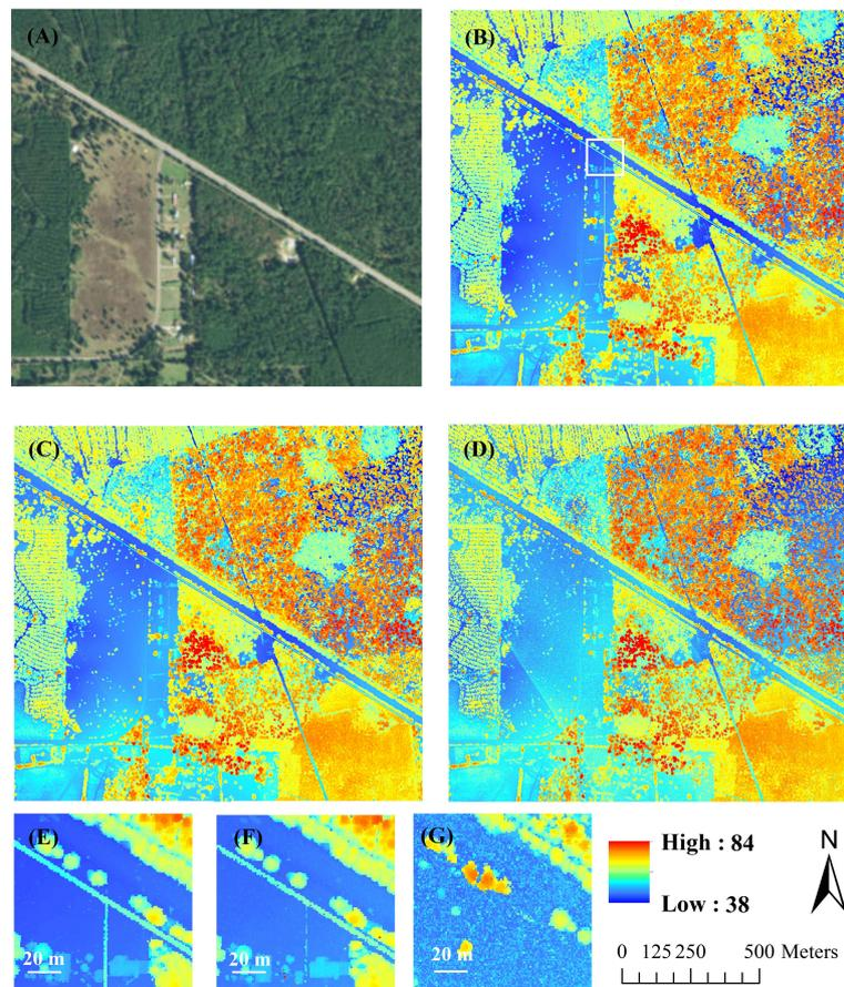
**Figure 9.** Satellite image and filtered single photon lidar results for the Lufkin area: satellite image of study area (A); VSAES result (B); AES only result (C); and DCC result (D). Detailed view of a portion of the powerline (E–G) corresponding to (B–D). The extents are labeled in (B) with a white square. The filtered results are colored by elevation.
