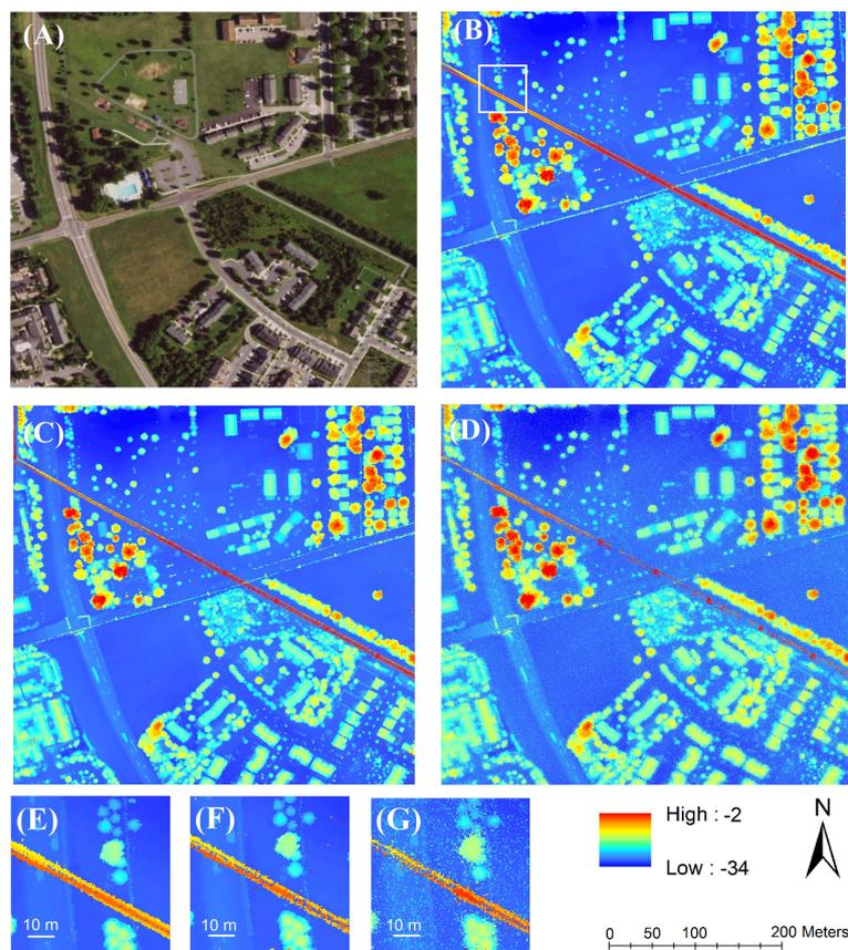
**Figure 5.** Satellite image and filtered SPL point clouds for the Easton study area: satellite image (A); VSAES result (B); AES only result (C); and DCC result (D). Detailed view of a portion of a powerline (E–G) corresponding to (B–D). The extents are labeled in (B) with a white square. The filtered results are colored by elevation.
