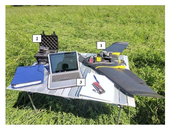
**Figure 2.** eBee Plus Unmanned Aerial Systems (UAS) platform and supporting ground control station for autonomous operations. Both the Sensor Optimized for Drone Applications (S.O.D.A.) (1) and multispectral Sequoia sensor system (2) integrated directly into the unmanned aircraft and were pre-programmed for specific image overlap in the eMotion3 flight planning software (3).
