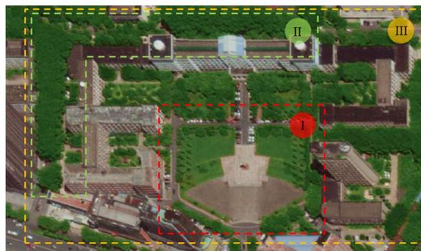
**Figure 6.** Study area. The three dashed boxes with different colors indicate different blocks for experiments. Blocks I and II were scanned with mobile laser scanning (MLS), while block III was scanned with airborne laser scanning (ALS) with a sparser point density.
