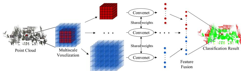
Figure 3. Multi-scale convolutional network.
