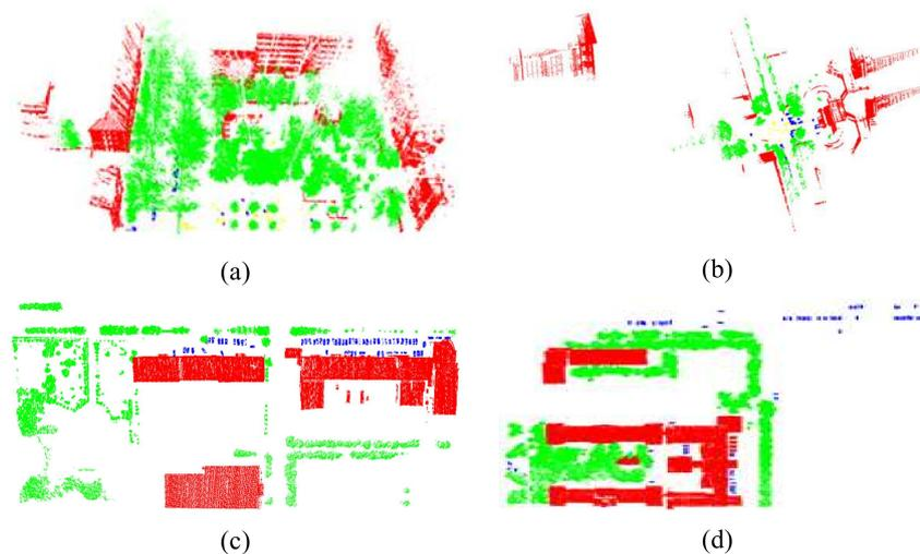
**Figure 11.** Ground truth of the terrestrial laser scanning (TLS-Wang) and ALS-Zhang point clouds. (a,b) are TLS-Wang scene I and II, while (c,d) represent ALS-Zhang scene I and II respectively.
