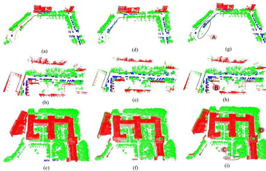
**Figure 8.** Classification results of test data. The first column shows the ground truth of the test data of blocks I, II, and III; the second column represents the predicted classification result without global label optimization; and the third column is the corresponding classification result with the proposed method. A, B, C, and D of the last column represent the typical cases that were mistakenly classified.
