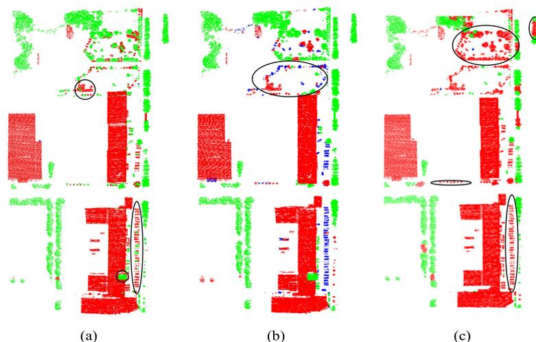
**Figure 14.** Classification results of ALS-Zhang scene I using MSNet trained with other data sets. (a–c) are the classification results using MSNet trained with the ALS-WHU, the ALS-Zhang scene II, and the MLS-WHU point cloud respectively.
