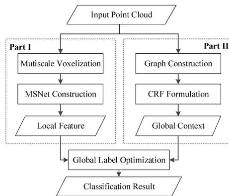
**Figure 1.** Flowchart of the proposed multi-scale convolutional network (MSNet).
