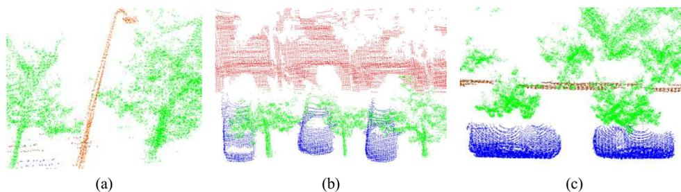
**Figure 9.** Details of some correctly classified objects. (a–c) show the lamp in the vegetation, the car with an incomplete shape, and the fence under the trees, respectively.
