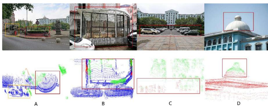
**Figure 10.** Actual situations corresponding to the typical cases that were mistakenly classified. The first row and the second row are the ground pictures and the point cloud details, respectively.
