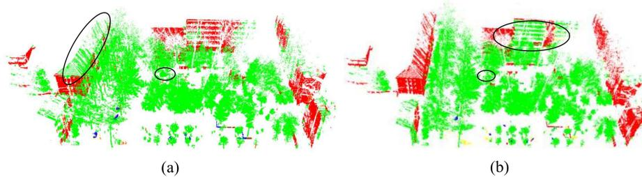
**Figure 13.** Classification results of TLS-Wang scene I using MSNet trained with other data sets. (a,b) are the classification results using MSNet trained with the MLS-WHU and the TLS-Wang scene II point cloud, respectively.
