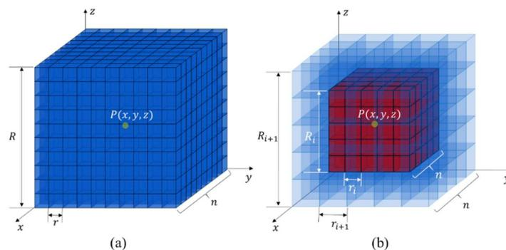
**Figure 2.** Point cloud voxelization at (a) uniform scale and (b) multiple scales. Around point  $P(x, y, z)$ , the spatial contexts of different sizes are partitioned as voxels of different scales, respectively. The points near  $P(x, y, z)$  are more important, and are characterized with finer scales in several voxels than those far away from it.
