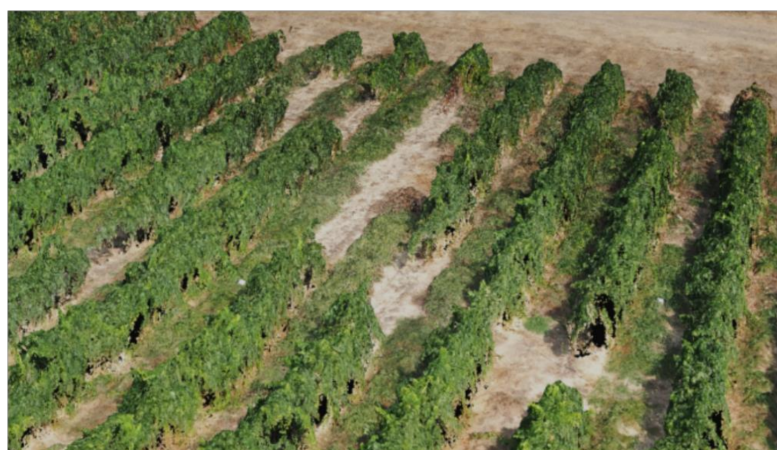
Figure 2. A partial view of the 3-D Point Cloud for the vineyard field A in July, which was produced by the photogrammetric processing of the remote images taken with the UAV.
