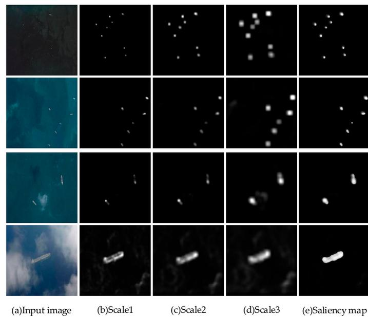
**Figure 4.** (a) A set of images containing the different size of targets; (b–d) Estimated saliency maps obtained at different scales (patch size parameter  $n = 4, 8, 16$  respectively); (e) Final saliency map based on the multi-layer cellular automata described in the text. By performing multi-scale saliency, our model is robust in the presence of target size changes. In addition, it can pop out the targets accurately and suppress the cluttered background effectively.
