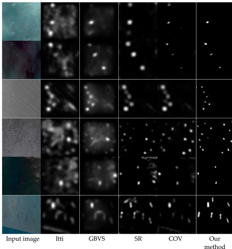
**Figure 8.** Examples of saliency maps with comparison to the 4 state-of-the-art methods. From left to right: input image, Itti [9], GBVS (Graph-Based Visual saliency) [10], SR (Spectral-Residual) [13], COV (Covariance saliency) [23], and our method. Our method outperforms other typical methods visually.
