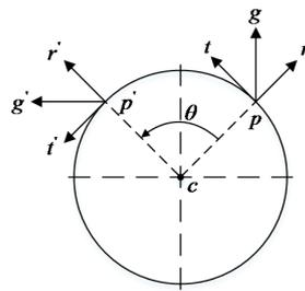
**Figure 6.** Illustration of radial gradient transform. For the given radial coordinate system  $(r, t)$ , when the chip is rotated by  $\theta$ , the projections of the gradient in  $(r, t)$  remain the same.
