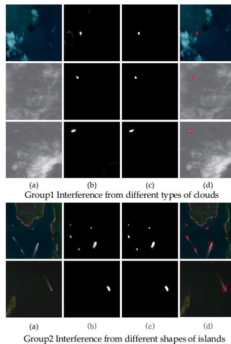
**Figure 5.** Candidate region detection results in complex backgrounds. Group 1 consists of images interfered by the cloud cover and group 2 consists of images interfered by islands. (a) Test image; (b) Saliency map generated by our visual attention model; (c) Image segmentation with Otsu algorithm; (d) Candidate region detection results.
