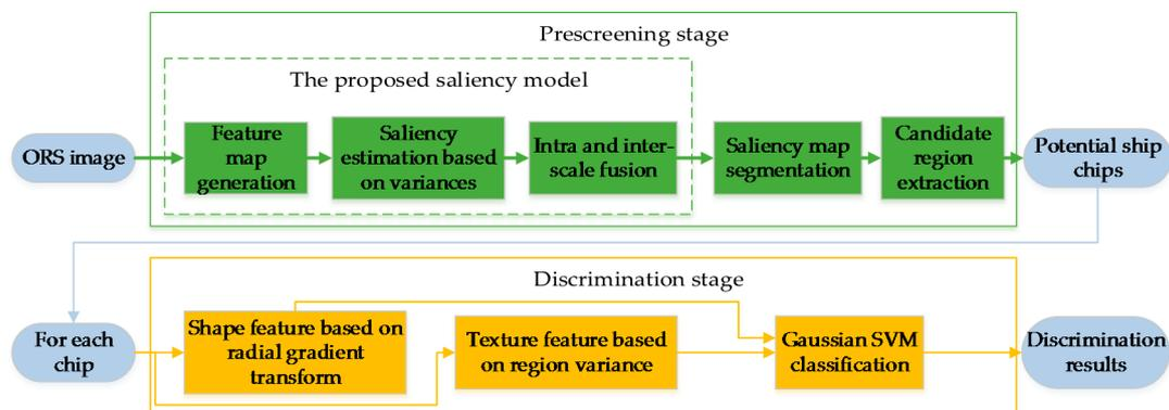
**Figure 1.** Diagram of the proposed hierarchical target detection scheme. The prescreening stage consists of saliency detection and binary segmentation. The discrimination stage includes feature extraction (radial gradient descriptor [19] and sigma set descriptor [20]) and classification by using Gaussian support vector machine (SVM) [21]. ORS: optical remote sensing.
