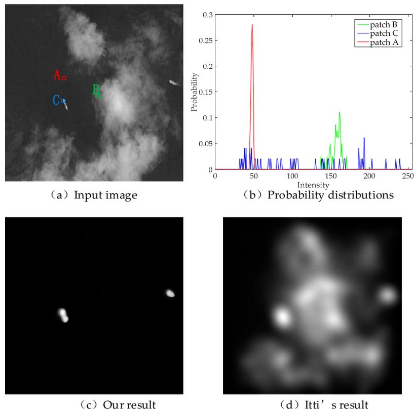
**Figure 2.** The proposed saliency model based on region variance analysis. (a) the original image; (b) probability distributions of patches A–C. The region variance values in terms of intensity information for A–C are  $2.8, 87.6$  and  $1.8 \times 10^3$ , respectively, and the sizes of A–C are all  $8 \times 8$  pixels. For contrast, our and Itti's results are shown in (c,d), respectively.
