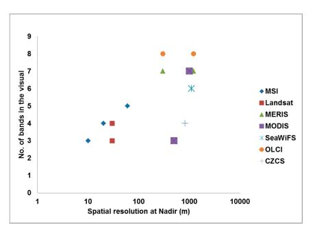
**Figure 1.** Plot of the available spectral bands in the visual range (400–710 nm) as function of spatial resolution for seven types of sensors. The multispectral imager (MSI) provides three different resolution modes, Landsat 8 has one band more than Landsat 7 at 30-m resolution. The Medium Resolution Imaging Spectrometer (MERIS), Moderate Resolution Imaging Spectroradiometer (MODIS) and Ocean and Land Colour Instrument (OLCI) provide products at two resolutions.
