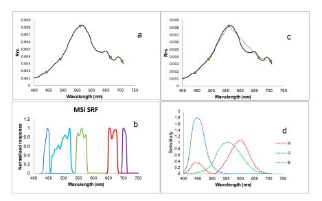
**Figure 3.** Original hyperspectral data plus green squares at the central positions of MSI bands (**a**); MSI measures the visual spectrum in only five wide bands (**b**); and the reconstructed spectrum will start to deviate from the original spectrum, especially at green and red wavelengths (**c**,**d**).
