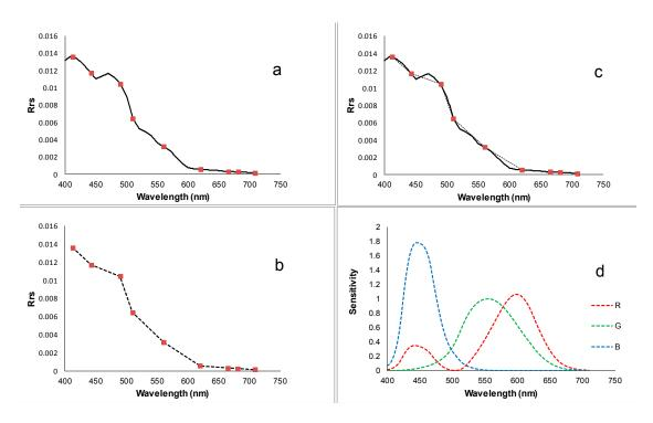
**Figure 2.** Original hyperspectral data plus red squares at the position of MERIS bands (**a**); the reconstructed spectrum from Rrs at nine MERIS spectral bands (**b**); a comparison of the two (**c**); and Colour Matching Function (CMF) curves for red, green, and blue that weight the spectral information to derive the hue angle (**d**).
