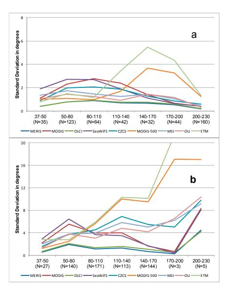
**Figure 6.** Plot of the standard deviation in the parameter ( $\alpha$ -sensor minus  $\alpha$ -hyperspectral) for nine sensors. On the horizontal axis, the hyperspectral hue interval is given in degrees, together with the number of spectra (N) that were used to calculate the standard deviation. The upper panel (**a**) is based on the International Ocean Colour Coordinating Group (IOCCG) data, and the lower panel (**b**) is based on the field data.
