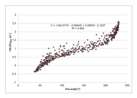
Figure 8. Relation between the hue angle and the absorption (a) of radiation at 440 nm.
