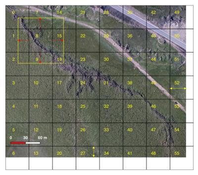
**Figure 5.** The grid for subdividing a sub-image (same as Figure 3c). The yellow number in each black square is the ID of the subdivided image patch. The yellow square is an example showing how we extend the boundary of a subdivided image patch (#8) from the black square to the yellow square. The yellow arrows in #52 and #27 indicate the patch width and height, respectively.
