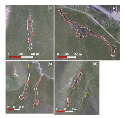
**Figure 8.** Zoomed-in comparisons between the gully polygons (red) and ground truth polygons (white). The yellow ones are false positives (same as in Figure 7). The extents of (**a**)–(**d**) are marked in Figure 7. See more discussion in Sections 5.2 and 5.3.
