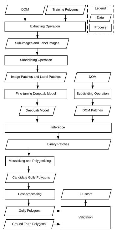
Figure 4. Flowchart of our mapping method based on DeepLab.
