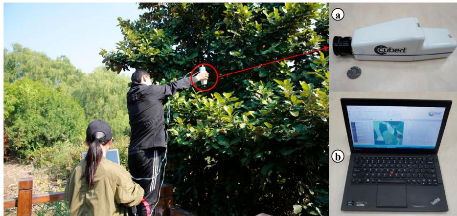
**Figure 3.** Field hyperspectral measurements above the mangrove canopies and the set-up used to acquire the hyperspectral images. (a) The UHD 185 hyperspectral imaging sensor, and (b) a notebook computer.
