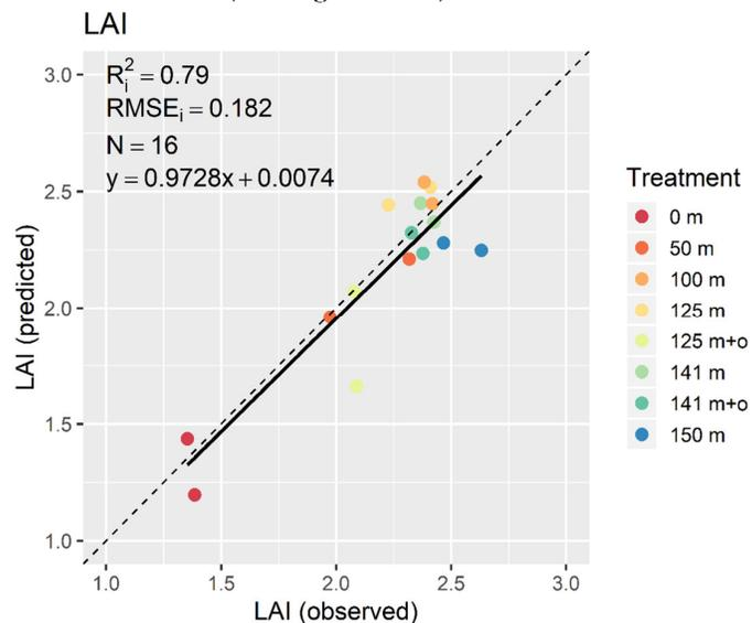
**Figure 7.** Scatterplot of independently validated partial least-squares regression (PLSR) models for leaf area index (LAI) with the regression line (continuous) and the 1:1 line (dashed).
