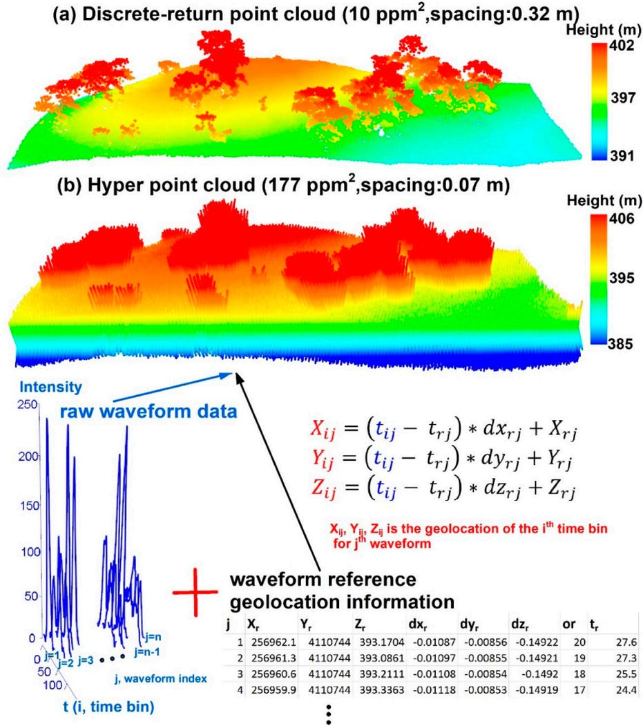
**Figure 3.** Comparison of the discrete-return LiDAR point cloud and the hyper point cloud (HPC) over the same subset region. (a) Discrete-return LiDAR point cloud. (b) Illustration of the HPC generation process by combing raw waveform data (blue) and corresponding waveform reference geolocation information (black).
