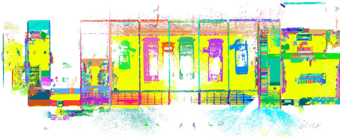
**Figure 12.** First level of Fire Brigade building. The amount of clutter and very large glass walls makes the process of wall detection challenging. The ceiling has two different heights and there is a lot of clutter below the ceiling. The colors represent the segments.
