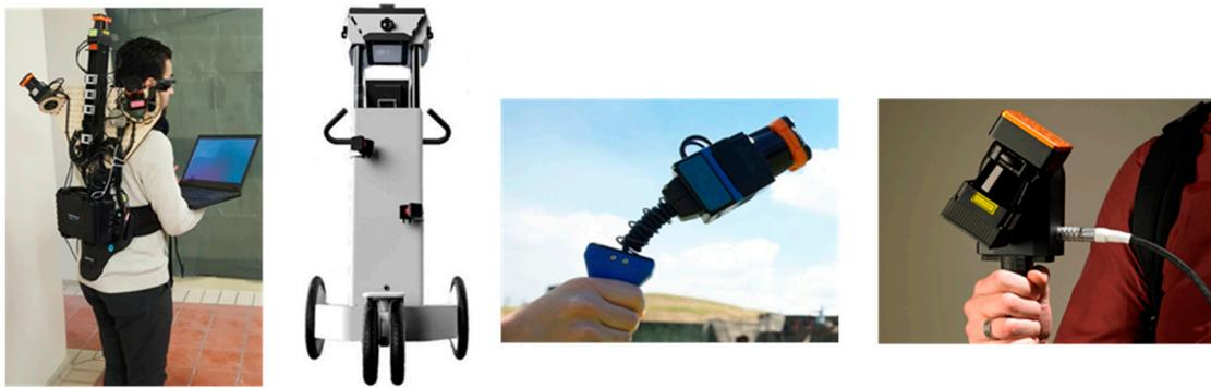
**Figure 1.** From left to right: Our prototype backpack system (ITC backpack), NavVis Trolley, Zeb-1 and Zeb-Revo.
