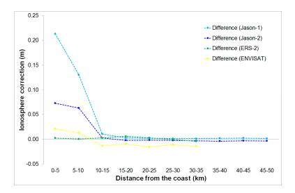
**Figure 7.** Difference between the ionosphere corrections from GIM and bi-frequency measurements for Jason-1 (light blue), Jason-2 (blue), and Envisat (yellow), and between GIM and Nic09 for ERS-2 (green) over La Rochelle within 50 km of the coast.
