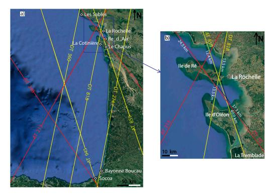
**Figure 2.** Google Earth image of the study area (**a**) with superposition of theoretical traces altimetry. Jason-1 and Jason-2 tracks are represented with red lines and ERS-2, Envisat, and SARAL tracks with yellow lines; (**b**) detail near La Rochelle tide gauge with Jason-1 and Jason-2 tracks in red lines and ERS-2, Envisat, and SARAL tracks in yellow.
