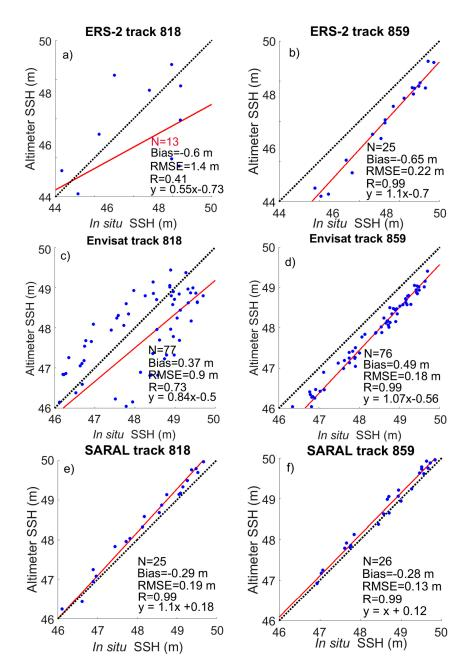
**Figure 4.** Comparisons between in situ and altimeter-based sea level anomalies in La Rochelle for (**a**,**b**) ERS-2; (**c**,**d**) Envisat; and (**e**,**f**) SARAL for descending track 0818 and ascending track 0859. The ionosphere and wet troposphere corrections were derived from GIM and ECMWF models, respectively.
