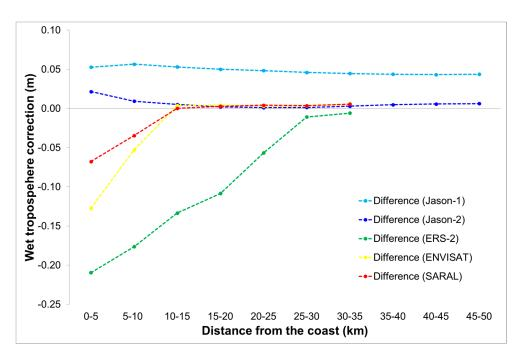
**Figure 10.** Difference between wet troposphere corrections from ECMWF and radiometer measurements for Jason-1 (light blue), Jason-2 (blue), ERS-2 (green), Envisat (yellow), and SARAL (red).
