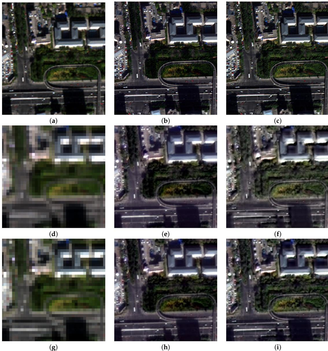
**Figure 6.** (a) Original multispectral (MS) image; (b) Fusion result of GS at full scale; (c) Fusion result of Indusion at full scale; (d) Degraded MS image by Aiazzi's method; (e) Fusion result of (d) by GS; (f) Fusion result of (d) by Indusion; (g) Degraded MS image by MSD4FV; (h) Fusion result of (g) by GS; (i) Fusion result of (g) by Indusion;
