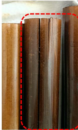
**Figure 5.** Specimen cracked due to sudden change of temperature.
