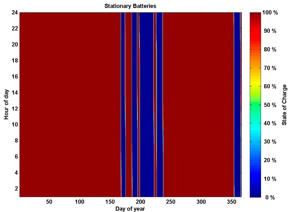
**Figure 1.** State of charge of stationary batteries. The utilization of stationary batteries by EnergyPLAN seems at odds with how such energy storage devices would be used in reality. EnergyPLAN used stationary batteries as a storage of lowest priority, while future prosumers may use them with the highest priority.
