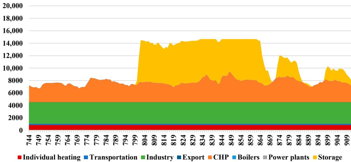
Figure S4. Grid gas demand (MW<sub>gas</sub>): February 1-7. Demand for gas in thermal power plants is high during the study period. Excess gas production is allocated to storage.
