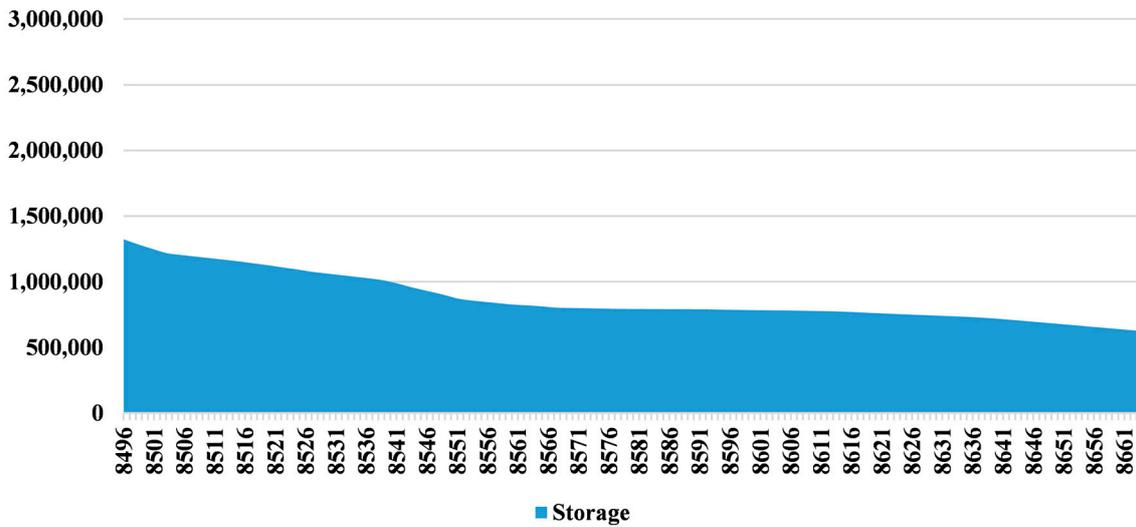
Figure S18. Grid gas storage ( $MWh_{gas}$ ): December 20-26. Maximum storage is 3 800 000  $MWh_{gas}$ . Grid gas storage is at relatively low levels for the year due to high demand. Storage levels decrease smoothly, however, due to variable production of synthetic methane from gasification of biomass and PtG.
