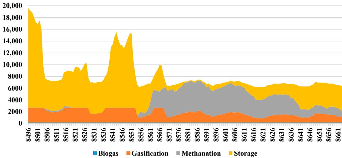
Figure S17. Grid gas supply ( $MW_{gas}$ ): December 20-26. High grid gas demand is mostly provided by storage over the study period. Relatively high PtG methane production is utilized directly after midweek. Biomass gasification is relatively strong during this period of high gas demand.
