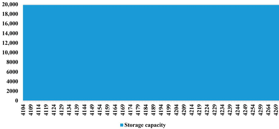
Figure S9. DH storage (MWh<sub>th</sub>): June 20-26. Maximum storage is 20 000 MWh<sub>th</sub>. Heat storage remains full throughout the study period due to very low demand for DH.
