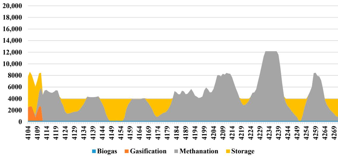
Figure S11. Grid gas supply ( $MW_{gas}$ ): June 20-26. PtG methane production corresponds to peaks in solar PV production during the study period. Gasification of biomass is unnecessary during most of the study period.
