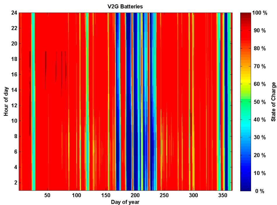
**Figure 2.** State of charge of V2G batteries. V2G batteries were a high priority storage solution for EnergyPLAN.
