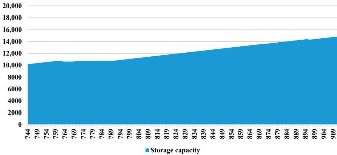
Figure S3. DH storage (MWh<sub>th</sub>): February 1-7. Maximum storage is 20 000 MWh<sub>th</sub>. Heat storage levels increase somewhat over the study period despite relatively high demands for heat. Power is a more limited commodity in the Finnish energy system. There appears to be an abundance of sustainable heat available throughout the year.
