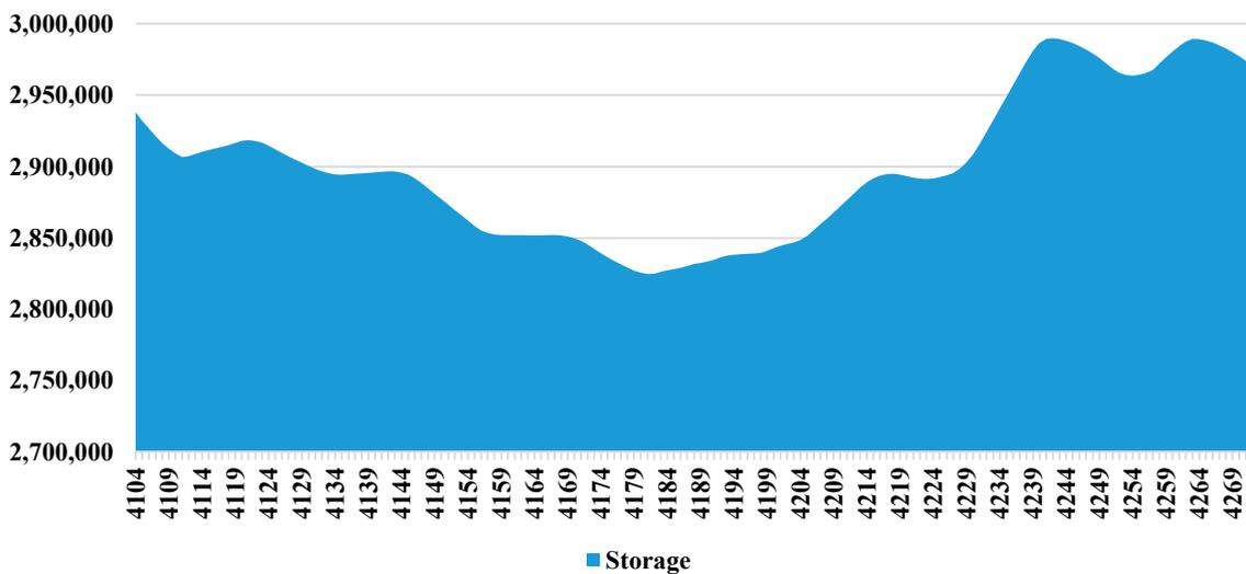
Figure S12. Grid gas storage ( $MWh_{gas}$ ): June 20-26. Maximum storage is 3 800 000  $MWh_{gas}$ . Small, daily increases in grid gas storage correspond to peaks in solar PV production. Small amounts of gas are used during the evening hours to produce power in CHP plants. Grid gas storage is close to maximum during the study period.
