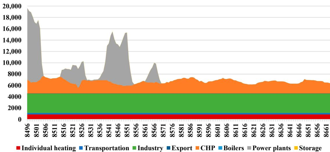
**Figure S16.** Grid gas demand (MW<sub>gas</sub>): December 20–26. Demand for grid gas in thermal plants is high during evening hours over the first half of the study period.
