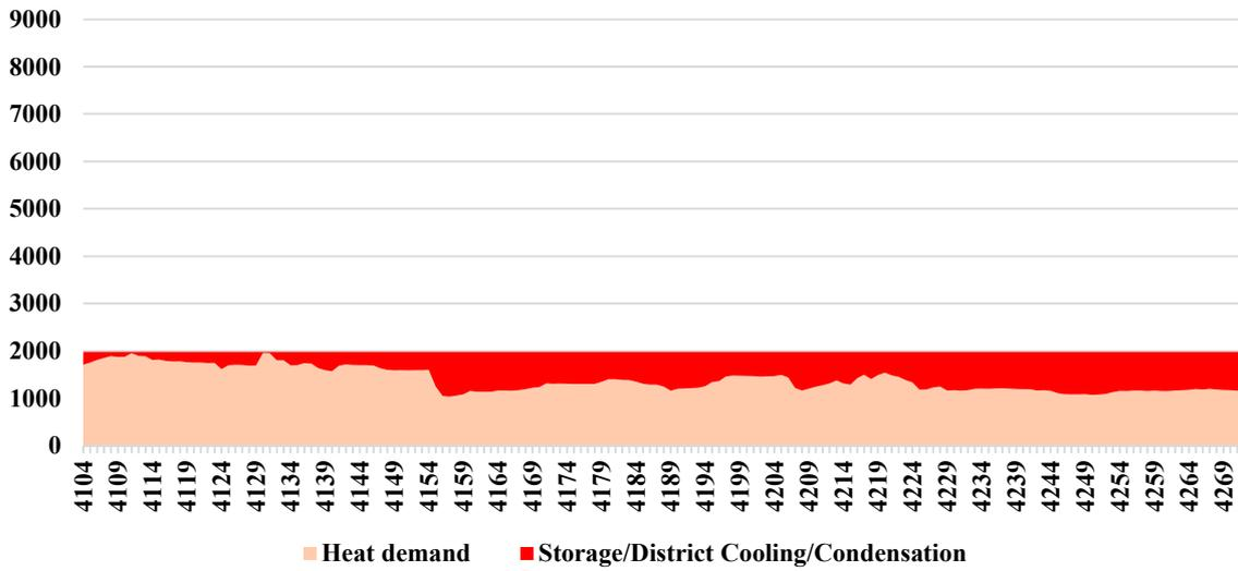
Figure S7. DH demand (MW<sub>th</sub>): June 20-26. Heat demand is low during the summer months. This study period also represents a time of reduced industrial heat use due to summer holidays. A significant amount of excess heat is therefore condensed.
