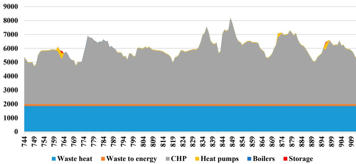
Figure S2. DH supply ( $MW_{th}$ ): February 1-7. CHP plants operate near maximum capacity during winter months. Waste heat is supplied from PtG as a constant source due to a limitation of EnergyPLAN. In reality, this heat production would be much more variable.
