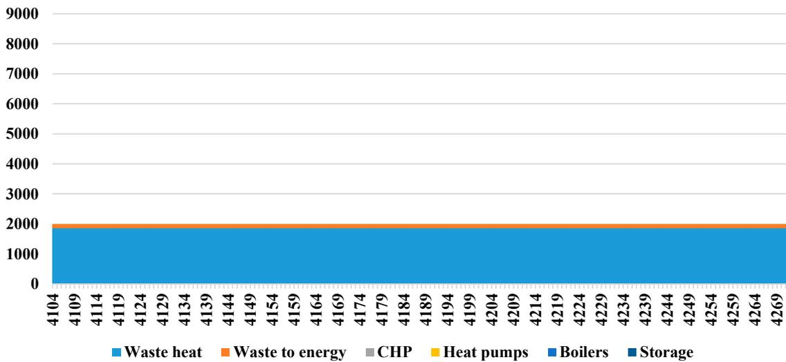
Figure S8. DH supply (MW<sub>th</sub>): June 20-26. Supply of heat mostly comes from waste heat resulting from the PtG process.
