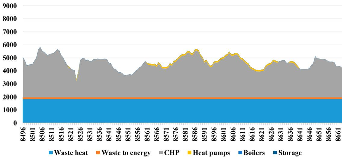
Figure S14. DH supply (MW<sub>th</sub>): December 20-26. CHP plants run at close to maximum capacity during this period. Colder temperatures during the mid-week necessitate the use of heat pumps for the DH system.
