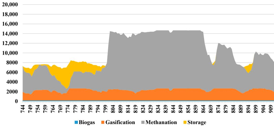
**Figure S5.** Grid gas supply ( $MW_{gas}$ ): February 1-7. Production of PtG methane is high during periods of high wind production during the study week. PtG production as occurs during noon solar PV production peaks. Gasified biomass also contributes to the gas grid during winter months.
