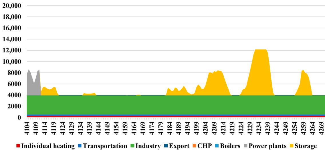
Figure S10. Grid gas demand (MW<sub>gas</sub>): June 20-26. Demand for grid gas is relatively low during the study period. Excess gas is allocated to storage.
