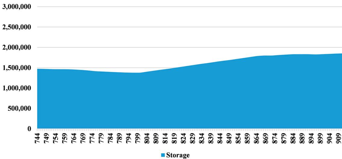
**Figure S6.** Grid gas storage ( $MWh_{gas}$ ): February 1-7. Maximum storage is 3 800 000  $MWh_{gas}$ . Storage levels of grid gas slightly increase during one of the weeks of highest gas demand due to high levels of PtG production that resulted from relatively high wind power production.
