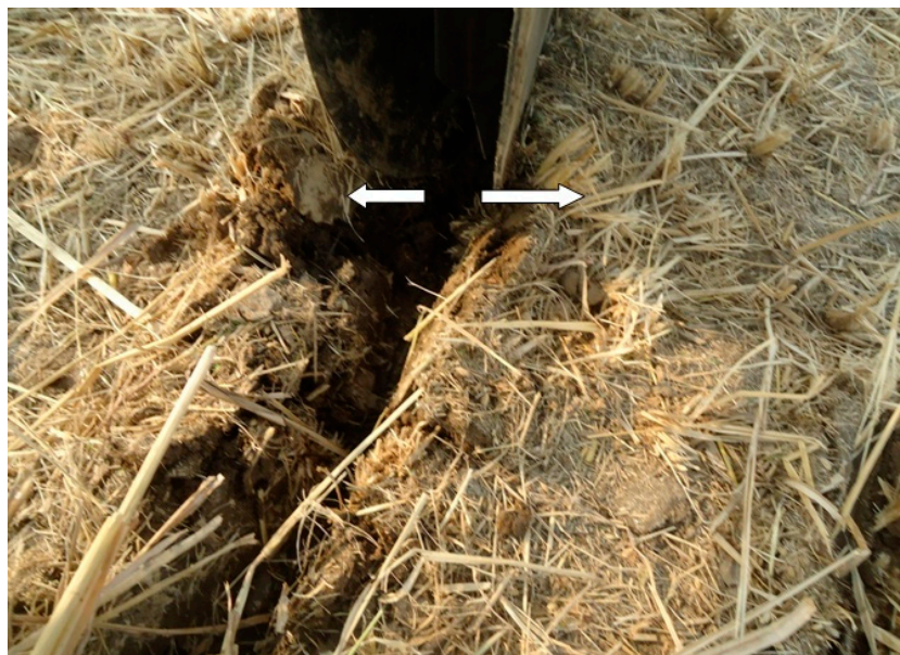
Figure 7. Soil failure and a furrow opened by a double disc opener.
