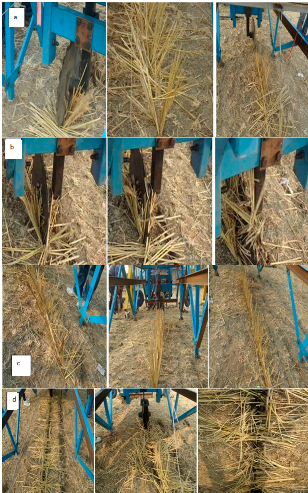
Figure 10. Straw cutting performance of (a) notched-type opener; (b) toothed-type; (c) smooth-type single disc; and (d) double disc furrow openers.
