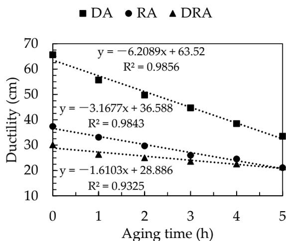
**Figure 4.** The ductility versus aging time of DA, RA, and DRA.
