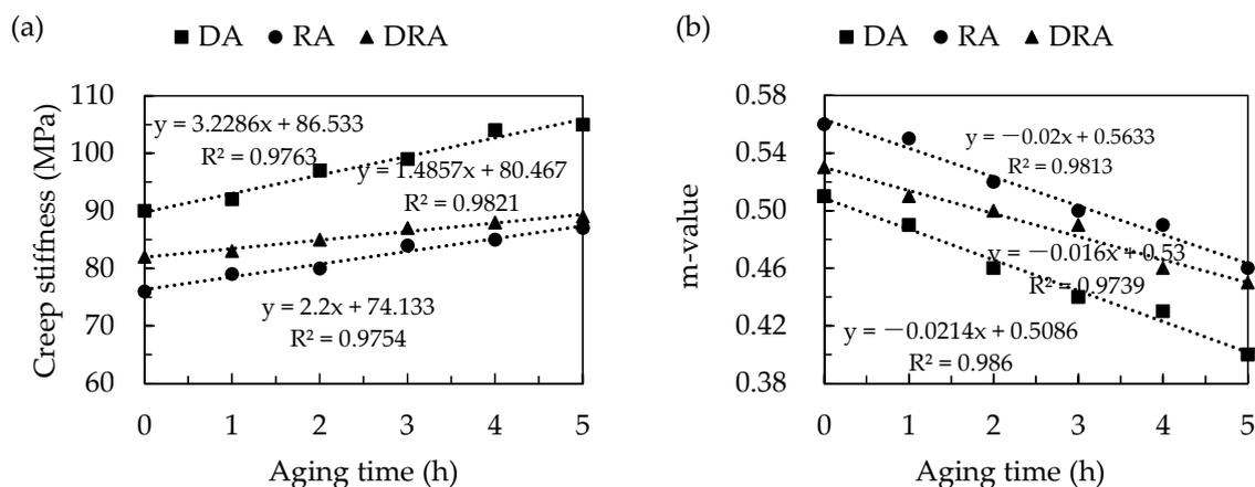
Figure 8. The creep stiffness and  $m$ -value versus aging time of DA, RA, and DRA; (a) creep stiffness, (b)  $m$ -value.
