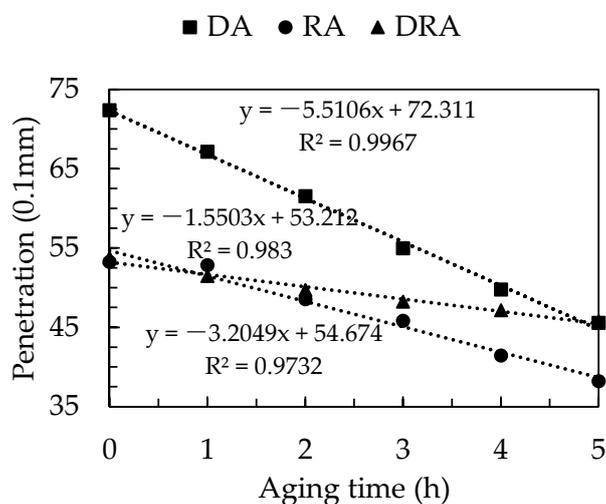
**Figure 2.** The penetration versus aging time of diatomite modified asphalt (DA), crumb rubber modified asphalt (RA), and diatomite and crumb rubber compound modified asphalt (DRA).
