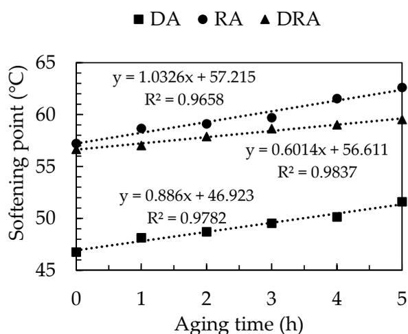
**Figure 3.** The softening point versus aging time of DA, RA, and DRA.
