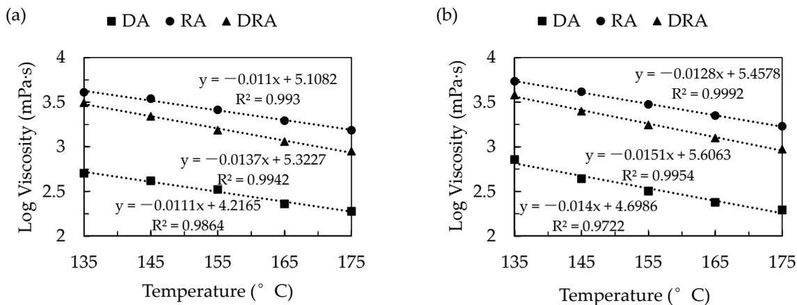
Figure 6. The viscosity versus temperature of DA, RA, and DRA (a) before TFOT and (b) after TFOT.
