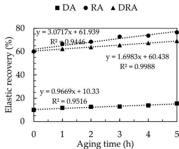
Figure 7. The elastic recovery versus aging time of DA, RA, and DRA
