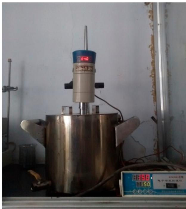
Figure 1. High speed shear homogenizer.
