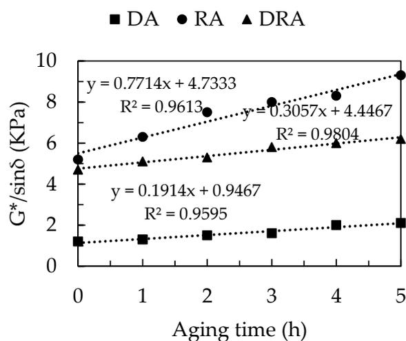
Figure 9. The rutting parameters versus aging time of DA, RA, and DRA.
