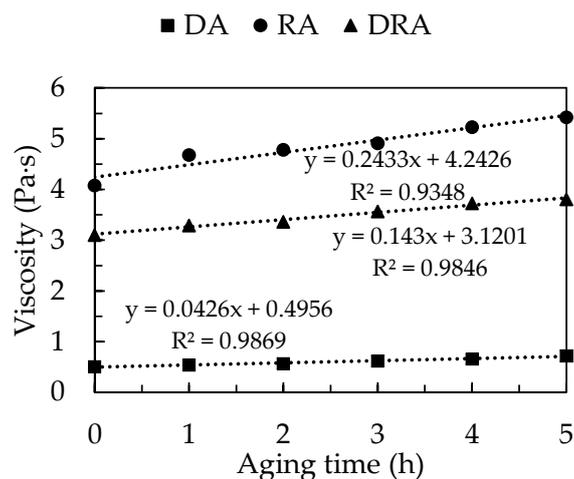
Figure 5. The viscosity versus aging time of DA, RA, and DRA.
