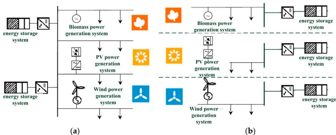
**Figure 4.** Micro-grid mode for rural electrification. (a) Hybrid micro-grid; (b) Independent micro-grid.
