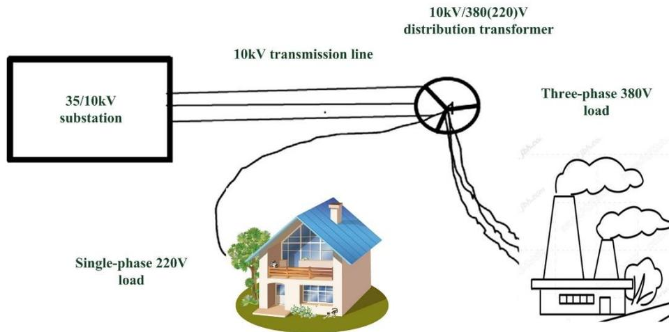
Figure 3. Schematic diagram of rural electrification by taking power grid extension mode.
