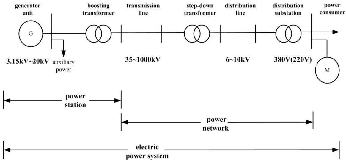
Figure 2. Schematic diagram of a generic portion of China’s electric power system.
