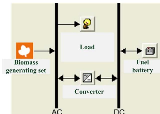
Figure 7. Biomass-based independent micro-grid system.
