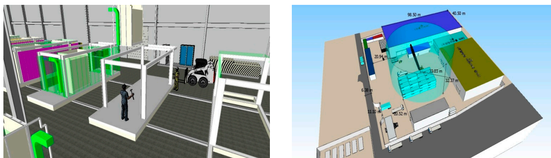
Figure 5. Manufacturing and installation plan for the factory/equipment linked UBR (left); and the yard storage plan for the manufactured modules (right).
