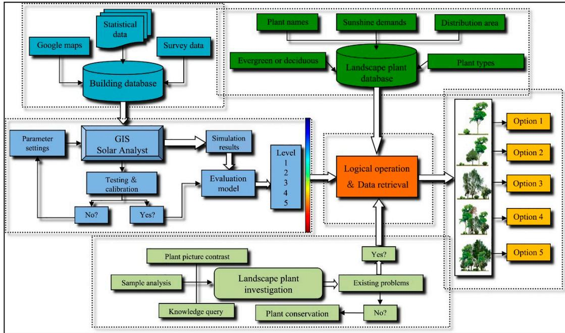
Figure 6. The workflow and technical route of Urban Plants Decision Support System (UP-DSS).
