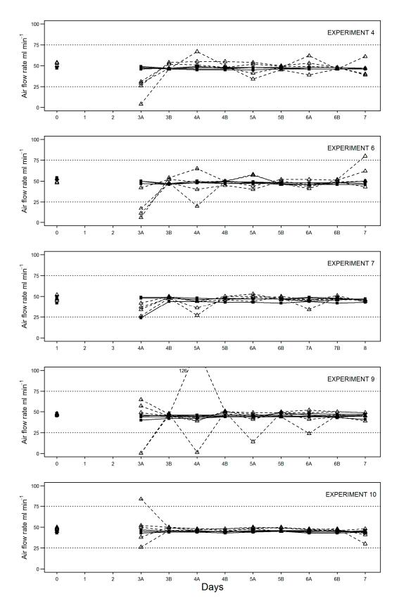
**Figure 3.** Air flow measurements from CO<sub>2</sub> collection vessel outlets in original (dashed line, open triangle data points) and modified (solid line, filled square data points) setups for experiments 4, 6, 7, 9 and 10. Replicate samples of each treatment are shown.
