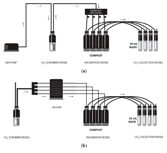
**Figure 1.** Schematic of the two ORG0020 setups; (**a**) original setup with diaphragm pump pushing air through  $CO_2$  scrubber and manifold delivering  $CO_2$  free air to vessels; (**b**) modified setup with multichannel pump pulling  $CO_2$  free air from a scrubber directly for individual vessels.
