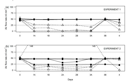
**Figure 2.** Air flow measurements from CO<sub>2</sub> collection vessel outlets in original (dashed line, open triangle data points) and modified (solid line, filled square data points) setups for (**a**) experiment 1 and (**b**) experiment 2. Four replicates of each treatment are shown.
