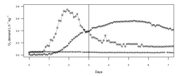
**Figure 4.** Oxygen demand of industry compost samples using modified DR4 respirometry, calculated as L  $h^{-1}$  kg<sup>-1</sup>. The vertical line separates the pre-incubation period (days 0 to 3) from the period recorded ORG0020 (days 3 to 7). Site D is indicated by open circle data points, site I by open diamond data points, and site G by open triangle data points.
