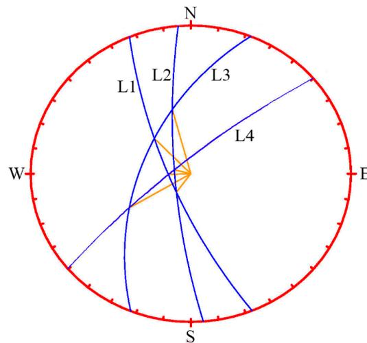
**Figure 2.** Main structure fissures stereographic projection.
