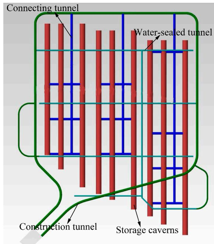
**Figure 1.** Layout plan of underground water-sealed petroleum storage depot.
