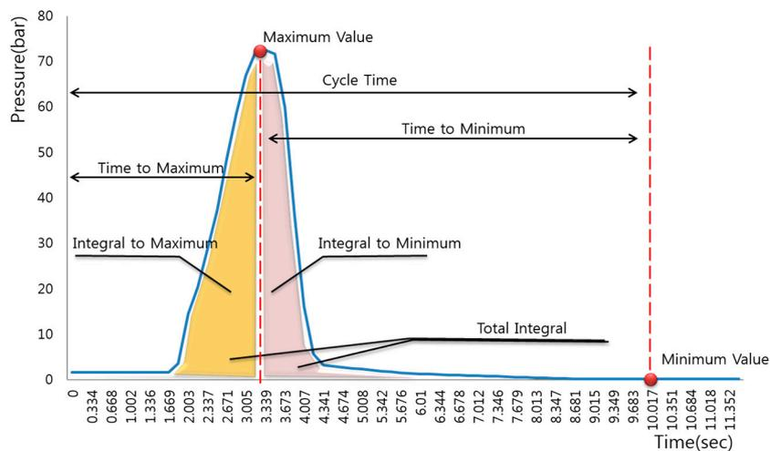
Figure 5. One set of features variable from injection pressure data.
