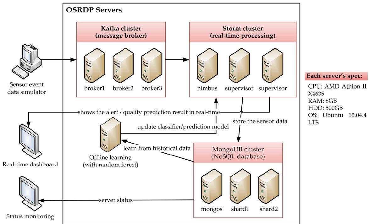
Figure 4. Configuration for simulation test.
