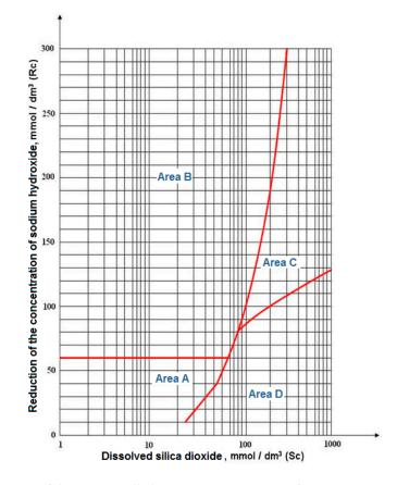
**Figure 3.** Verification of the reaction alkali–ggregates: aggregates from zone A are non-reactive and are recommended for utilization; aggregates from zone B are generally unreactive; aggregates from zone C are characterized by a potentially significant reactivity; and aggregates from zone D are considered harmful.
