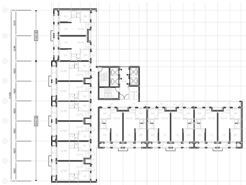
Figure 6. Case of computation of length ratio of bearing wall and column unit floor planning.
