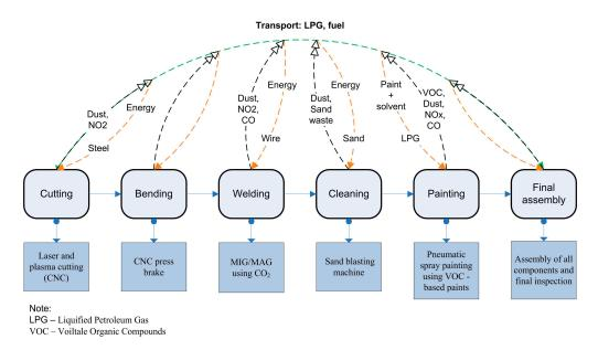
Figure 2. Environmental concerns associated with the process flow in boilers production for the baseline scenario.
