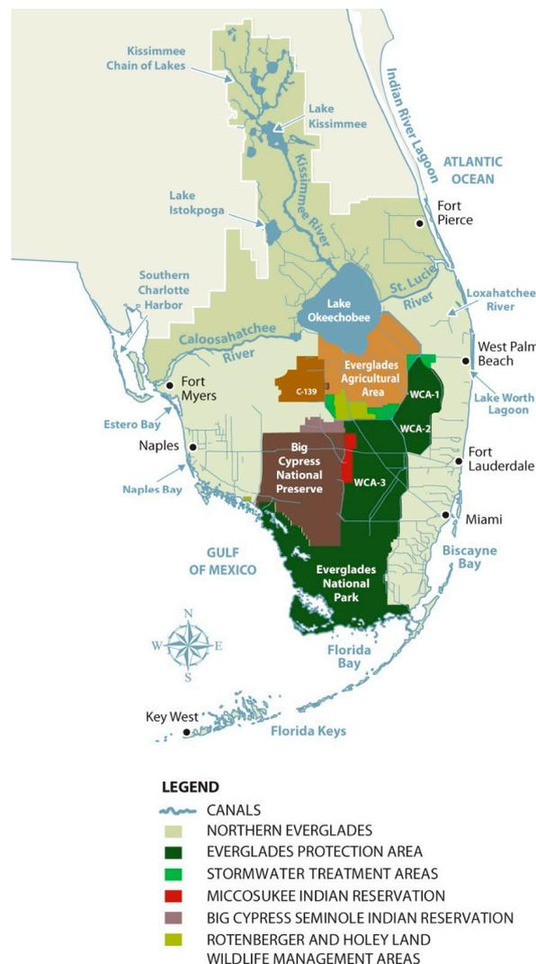
**Figure 3.** Compartmentalization of the present day managed Everglades ecosystem is broken up with the construction of levees, canals, and water control structures. Credit: South Florida Water Management District [25].
