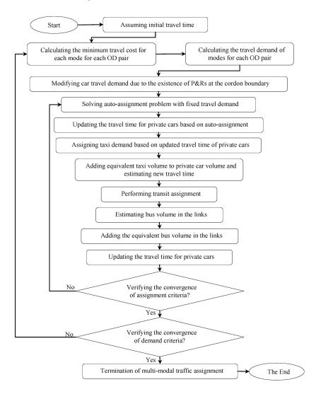
Figure 2. Solution algorithm for the lower level problem.
