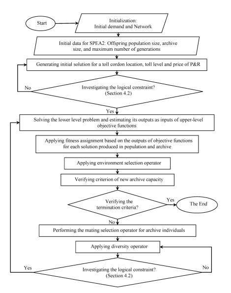
Figure 3. Algorithm for the solution of the developed model.
