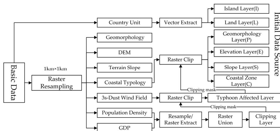
**Figure 3.** Flow chart of data preprocessing module. DEM represents Digital Elevation Model and GDP represents Gross Domestic Product. The clipping layer represents for the region of population density more than one person per  $\text{km}^2$  and GDP is more than \$50,000.
