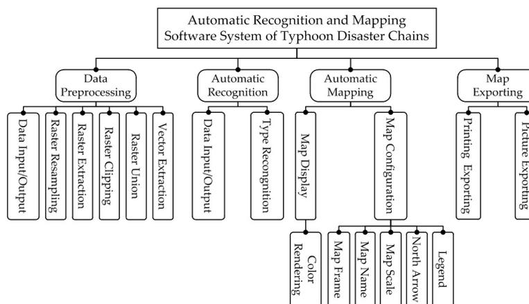
Figure 2. Framework of automatic recognition and mapping software system.
