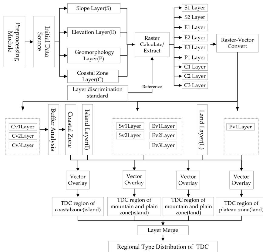
**Figure 4.** Flow chart of the automatic recognition module. TDC represents Tropical Cyclone disaster chains. The initial data used in the automatic recognition is provided by the preprocessing module.
